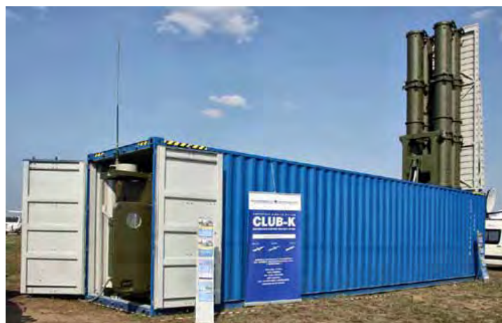
Figure 1. Russian CLUB-K cruise missile can be launched from a standard 12-meter shipping container, from [3].
