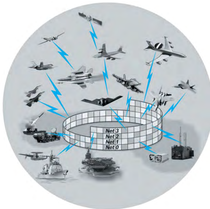
Figure 3. Link 16's ability to have simultaneous networks, from [10].
