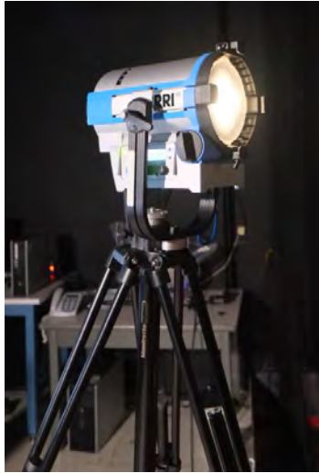
Figure 21. ARRI temperature lamp used in the FSS testbed to simulate changes in illumination conditions.
