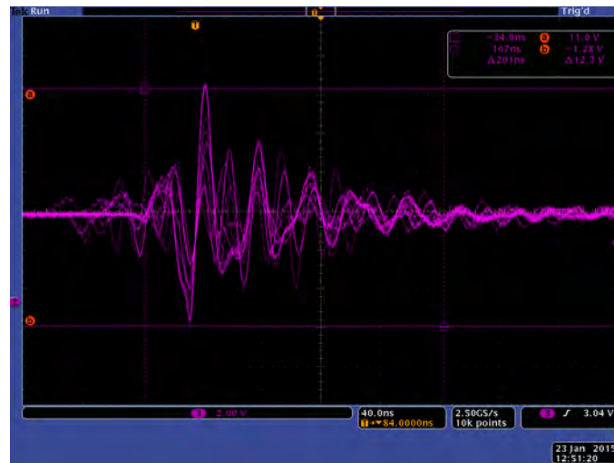
Figure 4.3. The voltage on the OD/\overline{SD} pin after increasing C_{SD} to 1000 pF. The time and voltage scale is 40 ns and 2 V per unit, respectively.
