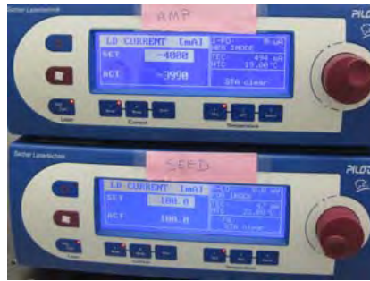
Figure 23. Seed and Amplifier max current settings for 1.94 Watt laser output
