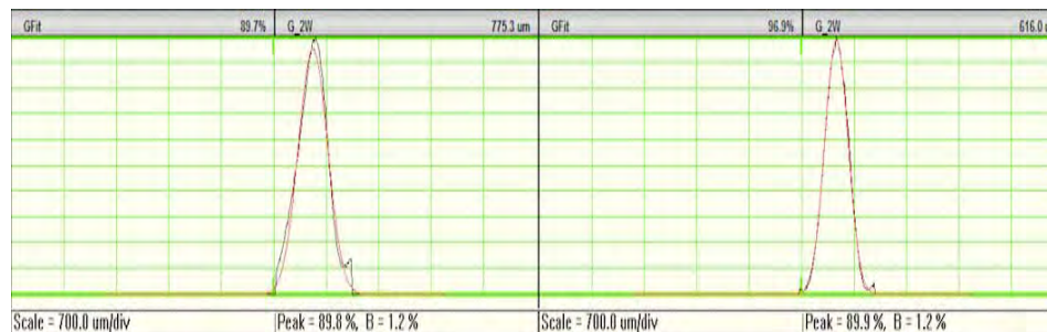
Figure 28. Orthogonal axis comparison for laser profile to Gaussian curve
