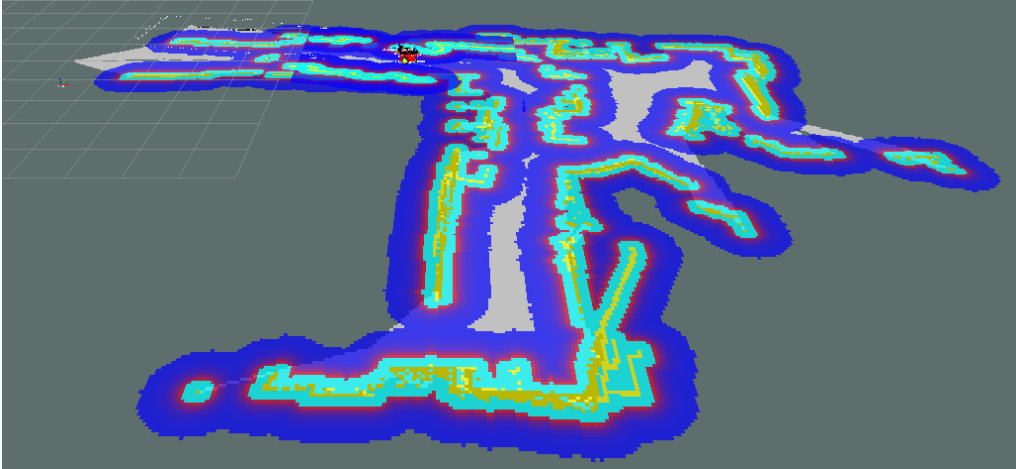
Figure 33. This image shows the global costmap while conducting autonomous navigation and SLAM of the interior of an office building.
