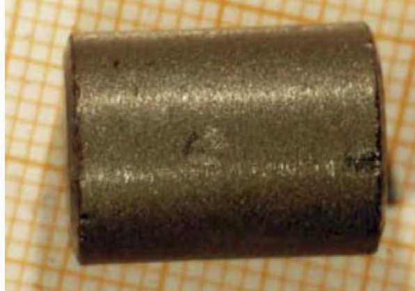
Figure 4. Uranium pellet from Find 1, from [4].
