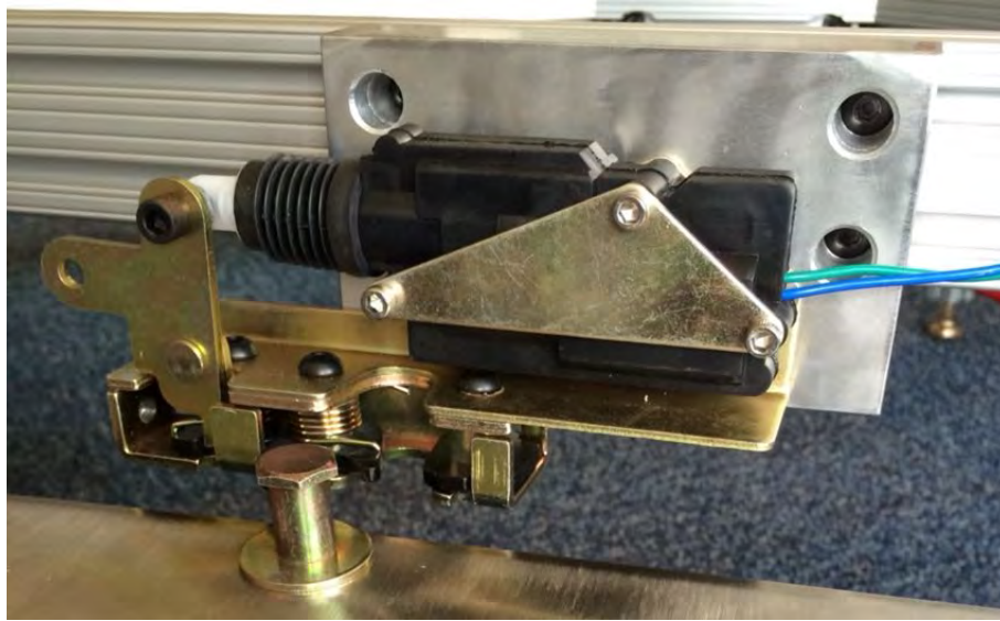
Figure 4.2: RULE mechanical holdback device, from [38]
