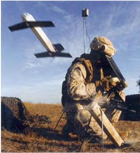
Figure 2.4: Tube launch of Army's Switchblade UAV, from [26]
