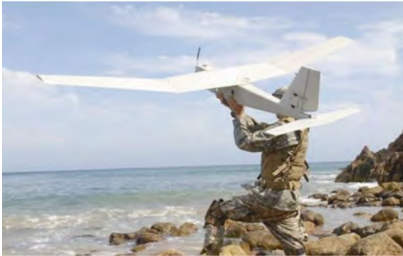
Figure 2.1: Hand launch of Army's Puma UAV, from [20]
