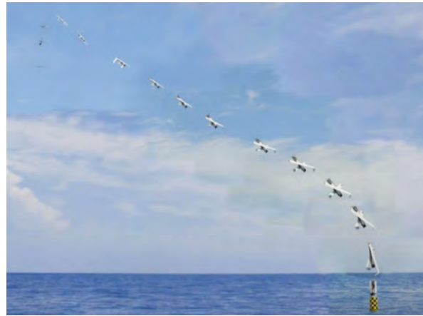
Figure 2.5: Underwater tube launch of an XFC UAV from a U.S. submarine, from [27]
