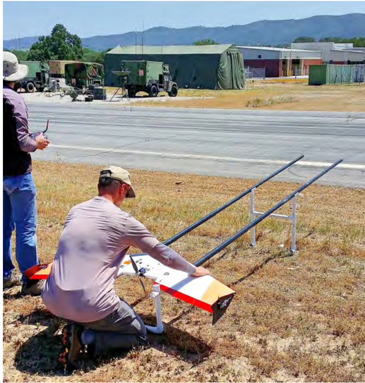
Figure 2.9: Naval Postgraduate School's ARSENL team launching a Zephyr II UAV using the bungee-operated launch system
