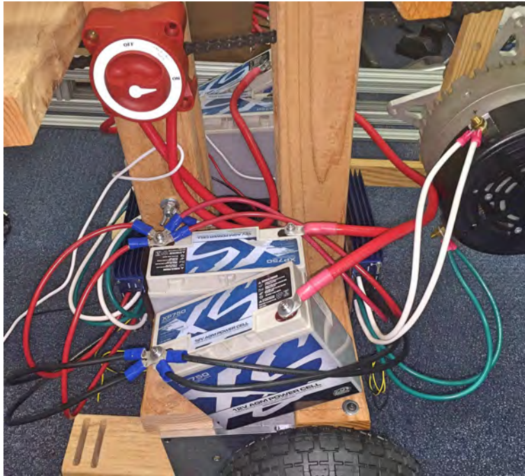
Figure 5.4: Electrical power kill switch for the chain launcher system
