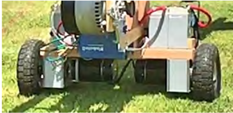
Figure 5.5: Chain Launcher wheel, motor, and gearbox assemblies mounted to underside of launcher frame
