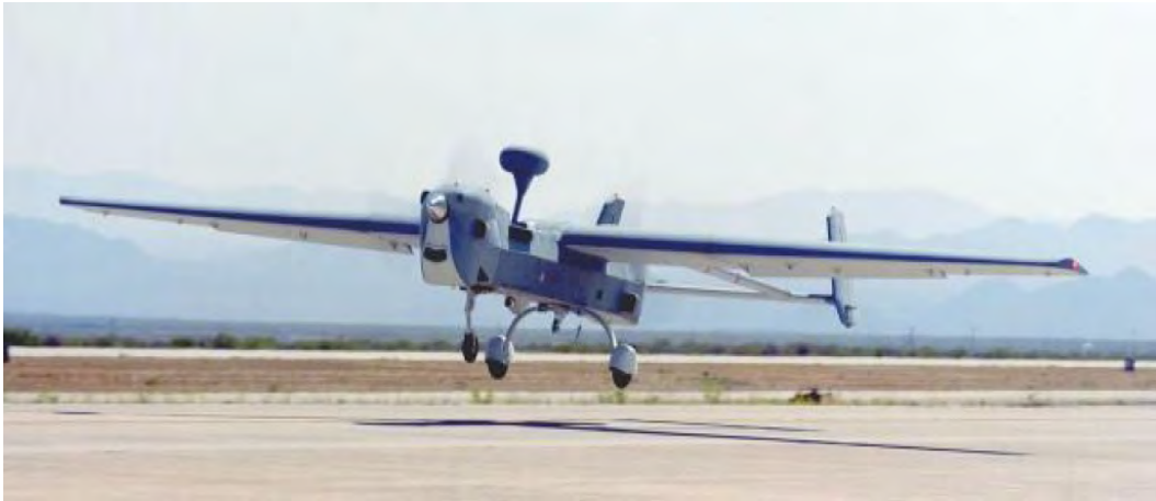
Figure 2.3: Conventional runway launch of Army's MQ-5 Hunter UAV, from [23]
