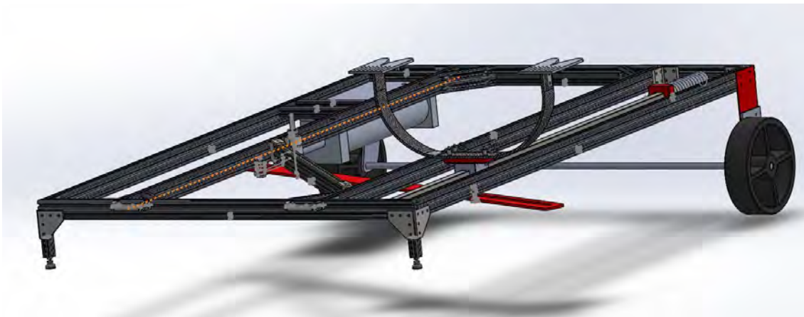
Figure 4.3: CAD drawing showing RULE's wheels and handles, from [38]
