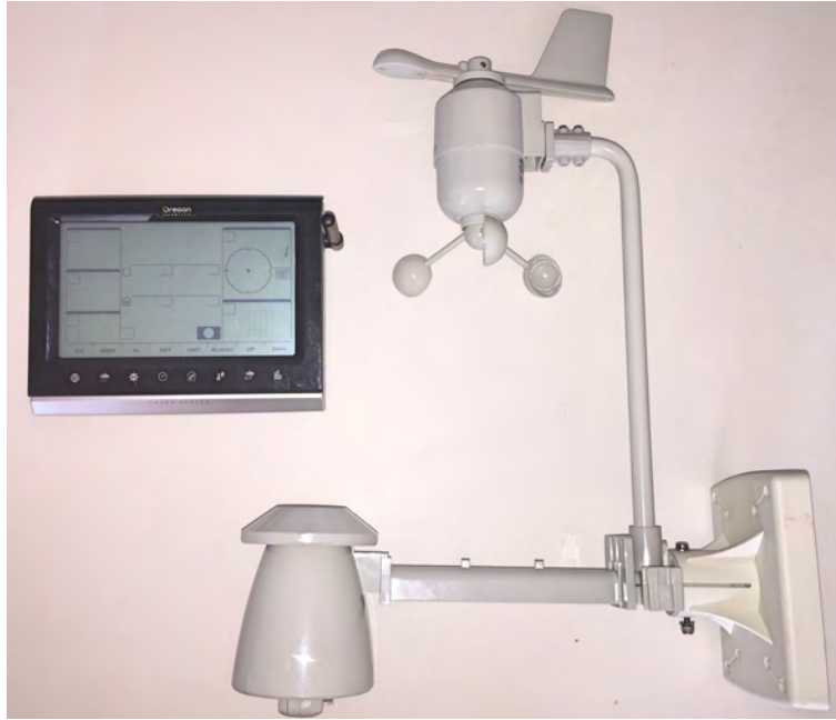
Figure 5.7: Oregon Scientific WMR200A Weather Station used to collect wind data
