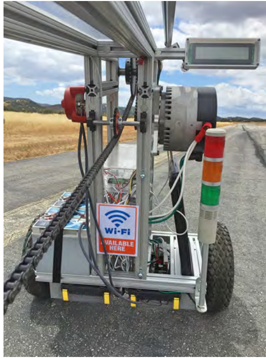
Figure 6.4: AMPPS status-indicating lighting system
