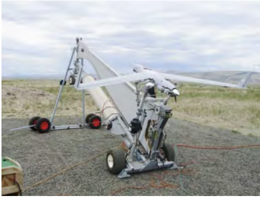
Figure 2.6: Pneumatic launch of Navy's ScanEagle UAV, from [28]
