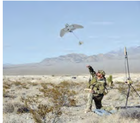
Figure 2.2: Hand launch of USMC's Wasp AE UAV, from [19]
