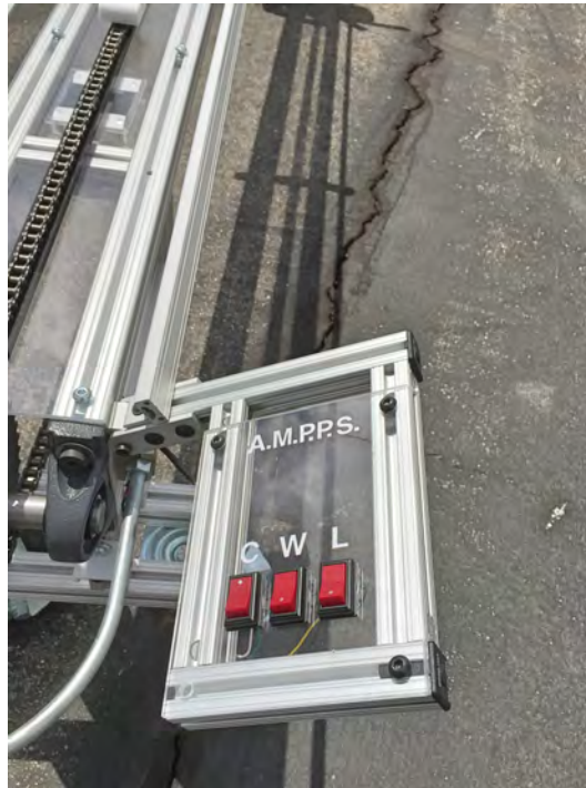
Figure 6.2: AMPPS mechanical-based system kill switches with easy operator accessibility
