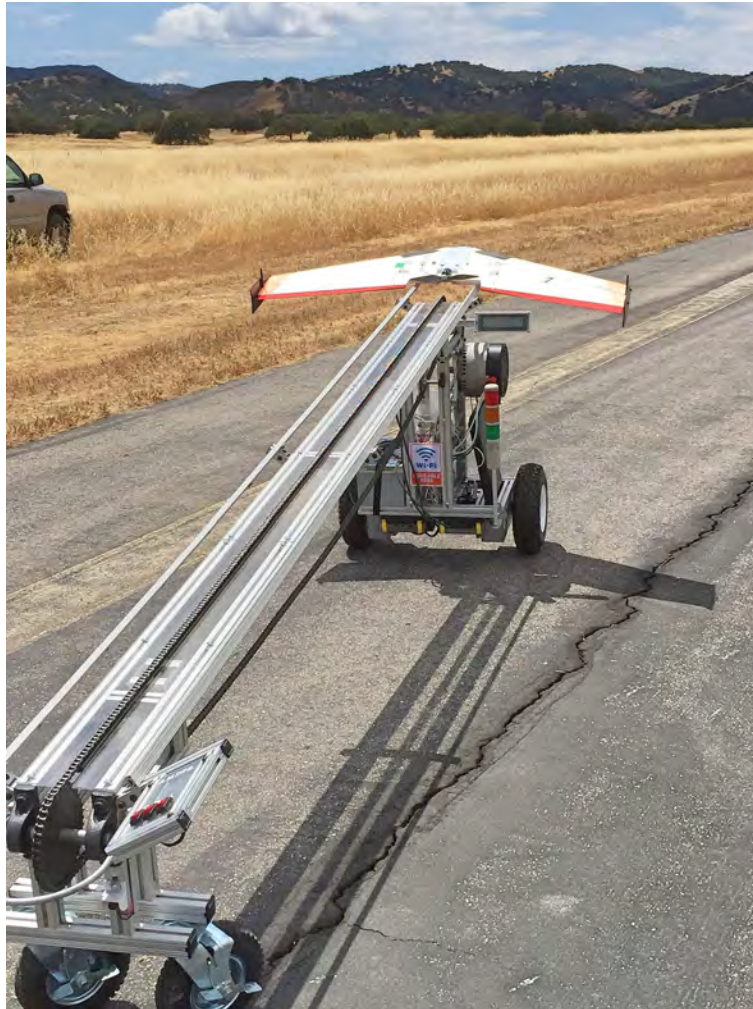
Figure 6.14: AMPPS demonstrating a successful UAV launch
