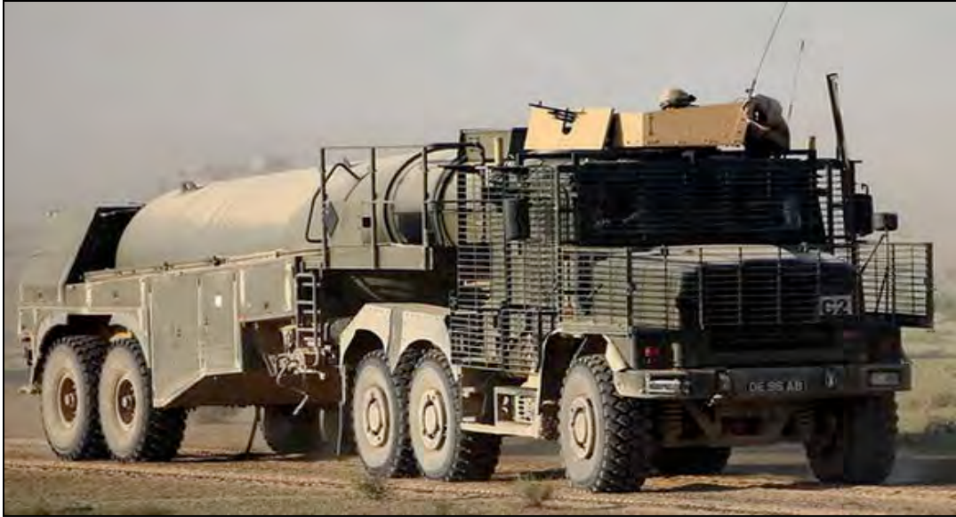
Figure 16. Oshkosh Wheeled Tanker (Medium Tactical Vehicle Replacement (MTVR) Mk 31 7-Ton Tractor Truck with Tank) (from Military-Today.com, 2015).
