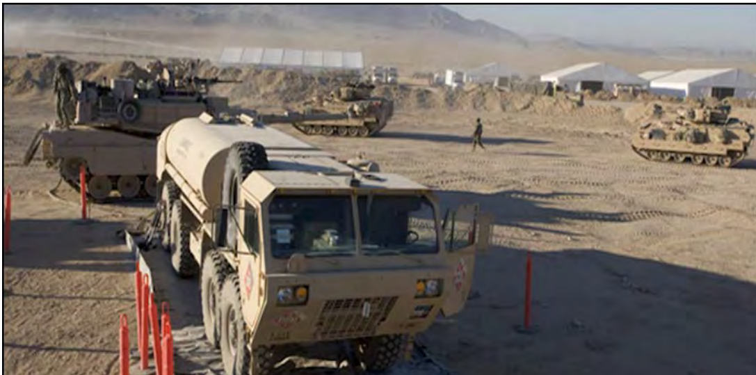
Figure 15. M978 A4 Heavy Expanded Mobility Tactical Truck (HEMTT); a 2,500-gallon tanker (from Basic Concepts Inc., 2015).
