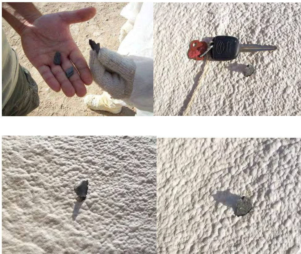
Figure 6. CCSF-sprayed military tent resists shrapnel penetration; October 17, 2008 (from Mason Knowles Consulting LLC, 2015).
