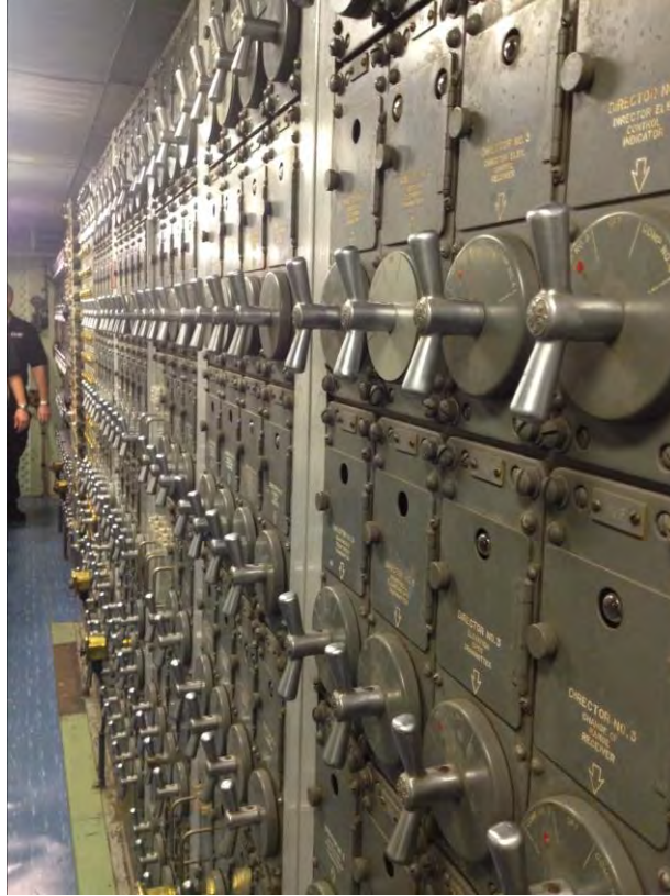
Figure 3. USS Missouri Fire Control Computer. The USS Missouri was commissioned in 1945 and was retired from service in 1992. This fire control computer was designed in 1941. The same type of computer for a modern-day ARLEIGH BURKE class Guided Missile Destroyer takes up a fraction of a commercial blade server rack (from Rumberg, 2013).
