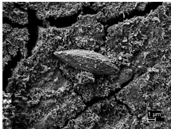
Figure 61. SEM images of aragonite crystal in low (left) and high (right) magnification
