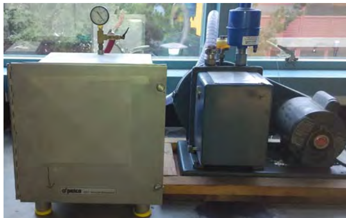
Figure 9. Vacuum chamber (on left) and dual-seal vacuum pump (on right) by Welch Manufacturing Co. (Chicago, IL)
