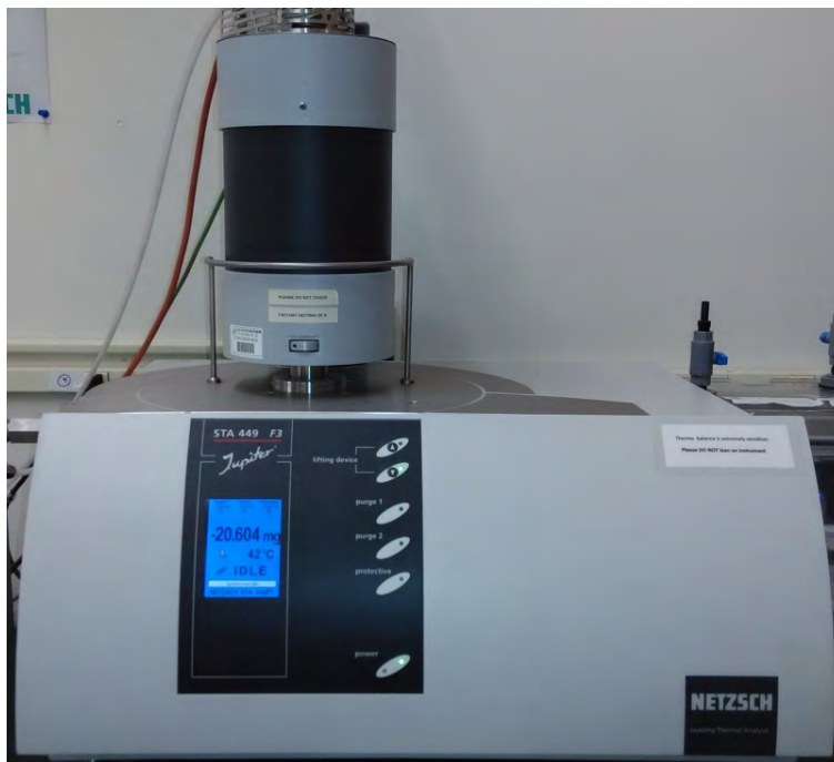
Figure 12. Diagram of NETZSCH STA 449 F3 Jupiter DSC/TGA (top) and picture of setup in NPS laboratory (bottom), from [43]
