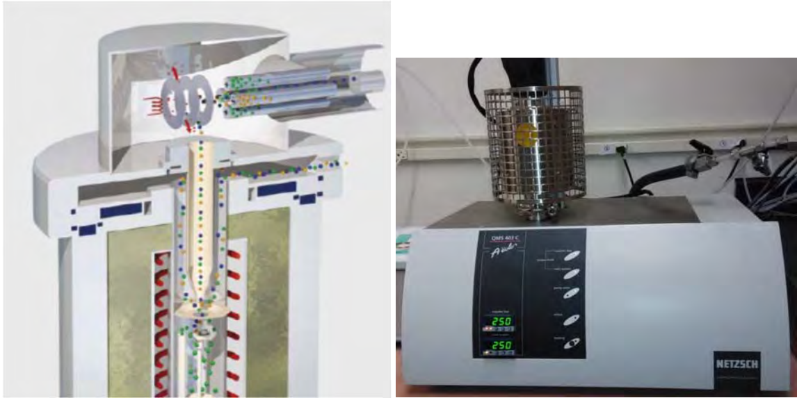
Figure 13. Diagram of NETZSCH TA-QMS 403C Aëolos QMS (left) and picture of setup in NPS laboratory (right), from [43]
