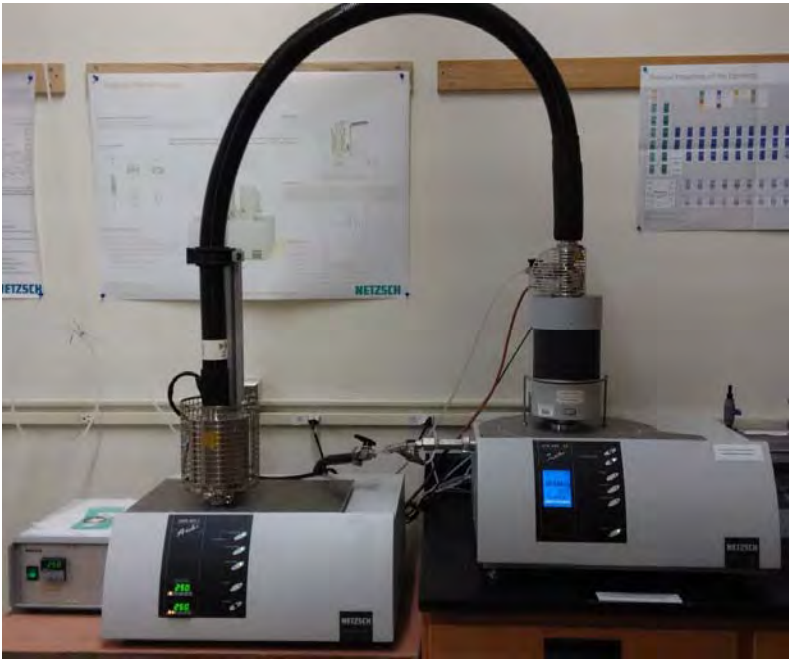
Figure 14. TGA/DSC coupled with the quadrupole mass spectrometer (QMS)
