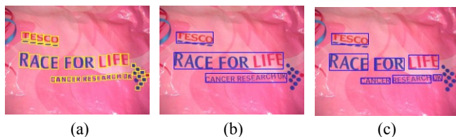
Fig. 5. (a) Connected components, (b) Text line bounding boxes, (c) Word bounding boxes
