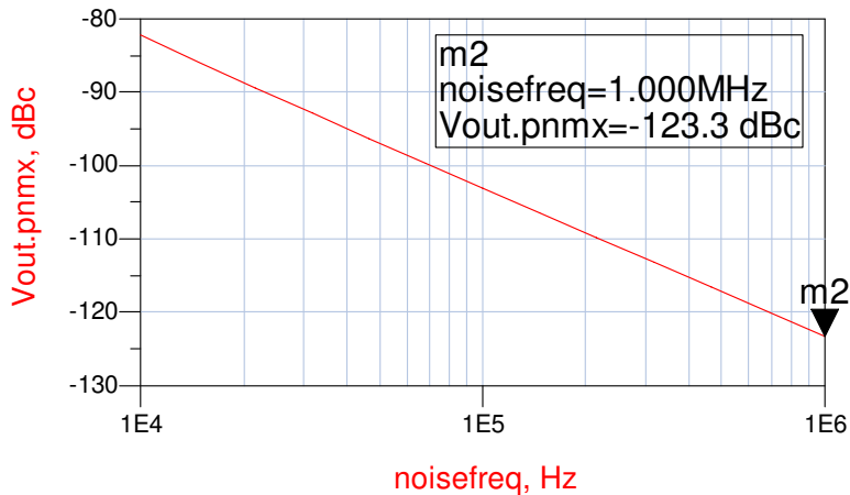
Figure 52: Simulated VCO phase noise with noise filtering in the current source
