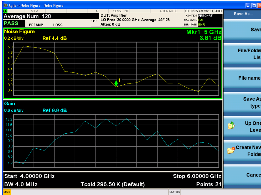
Figure 23: Agilent N9020A MXA Signal Analyzer screen shot for the noise figure measurement of LNA #1
