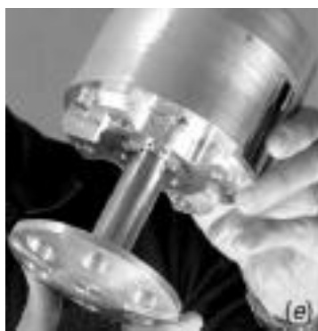
Figure 7 Piston of Sandia Hopper actuated through combustion of propane
