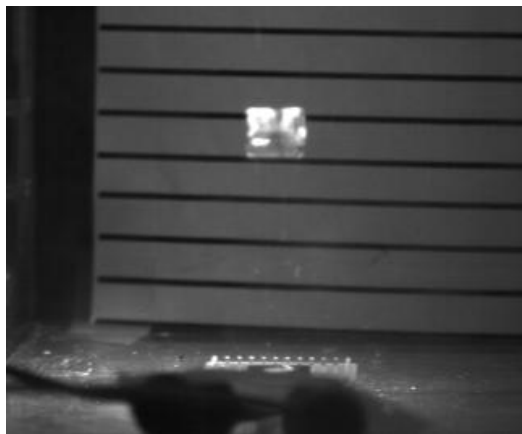
Figure 22 Thrust demonstrated to propel an aluminum foil flyer
