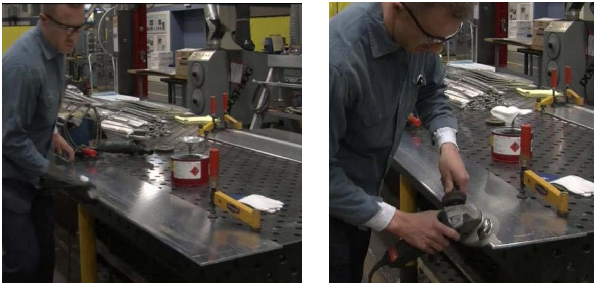
Figure 4 – Solvent Cleaning and Wire Brush Abrading of Plate Edges
