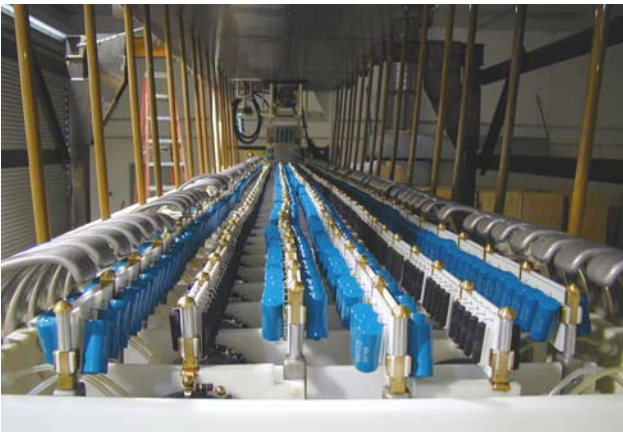
Figure 5. Top view of Marx showing charging and trigger resistors.
