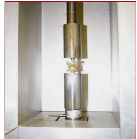
Round bar test in progress
