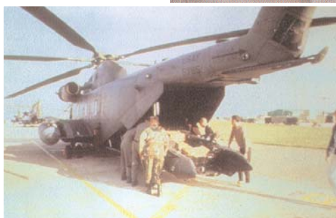
Securing soft duck boat on MH-53 helicopter.
