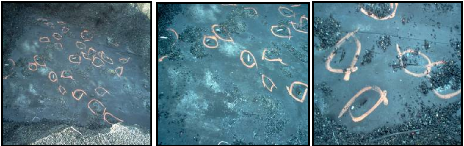
Range 5 (holes/tears circled, some with bullets protruding)
