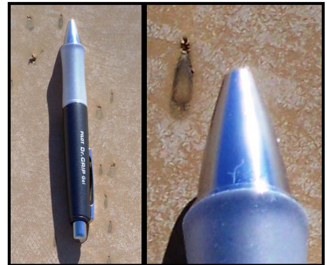
Marks and entry points on the top rubber cover caused by 5.56mm rounds
