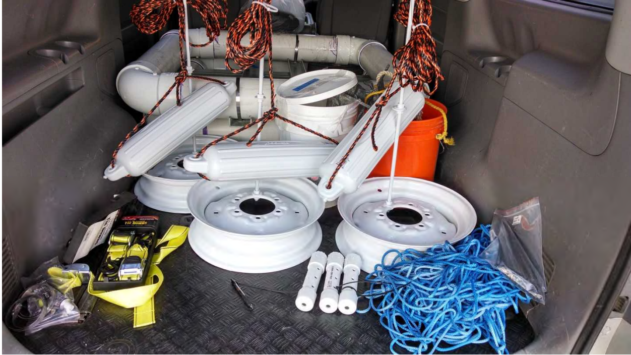
Figure 5-19. Rims used to anchor water level gauges. Pressure gauges were fixed to the vertical rods to be 30 cm above the sea floor.
