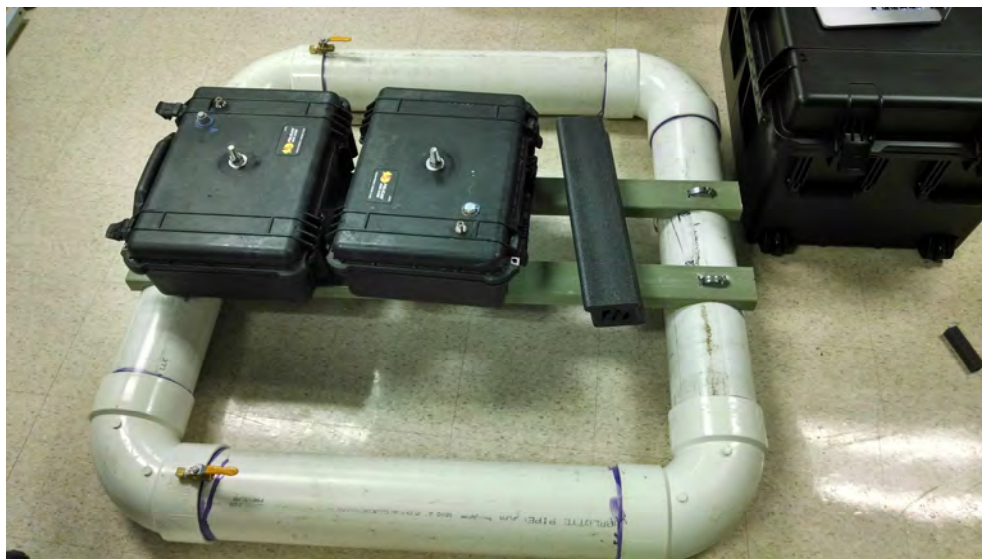
Figure 5-17. Water level buoy. Kinematic GPS unit being prepared in the black case mounted in the center.
