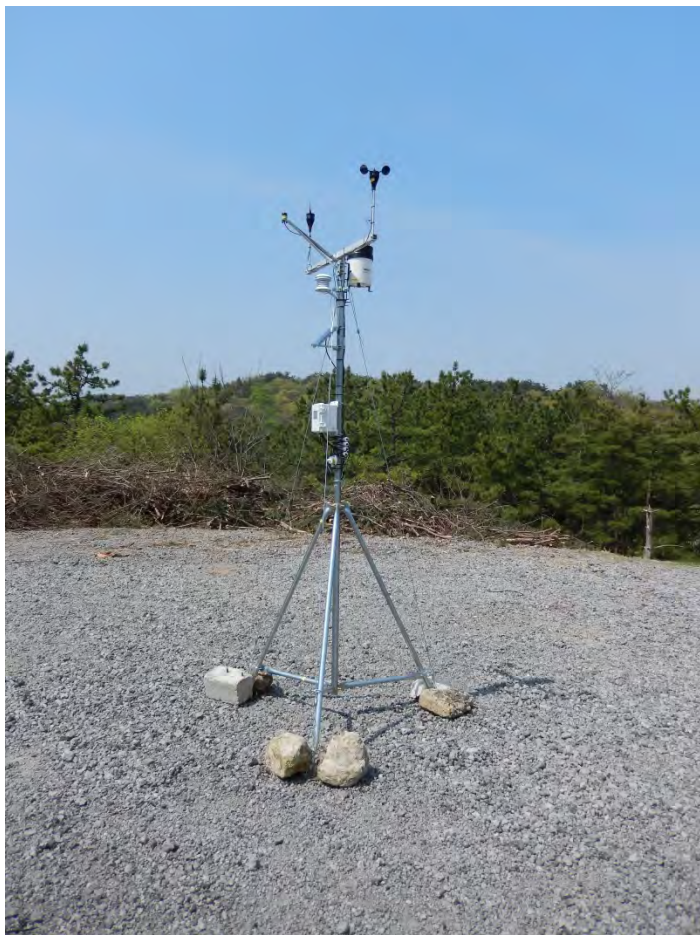
Figure I- 2. Meteorological Station Assembled at Camp Mujuk.
