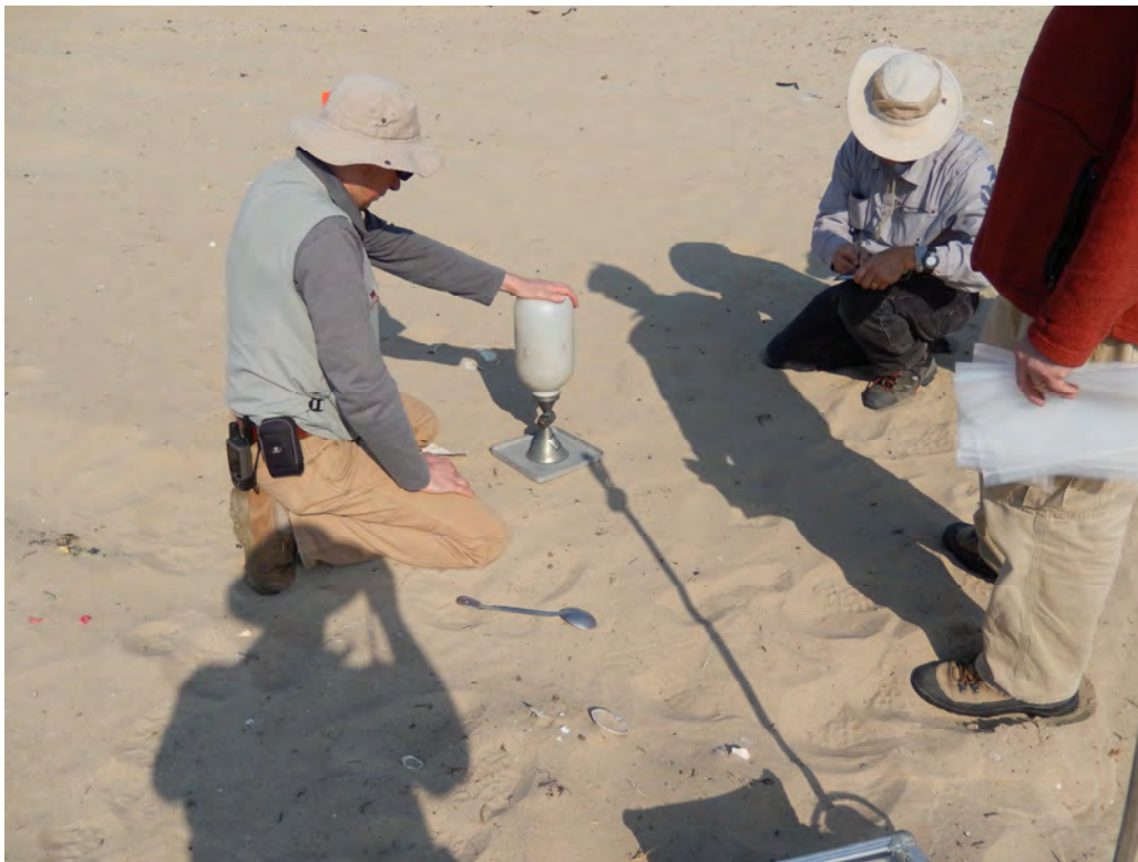
Figure 5-8. Sand cone density apparatus. Canister with calibrated sand is placed over the excavated hole (and a standard base plate) for determination of the wet field density of soil. Dry density is calculated after the laboratory measurement of the field moisture content.
