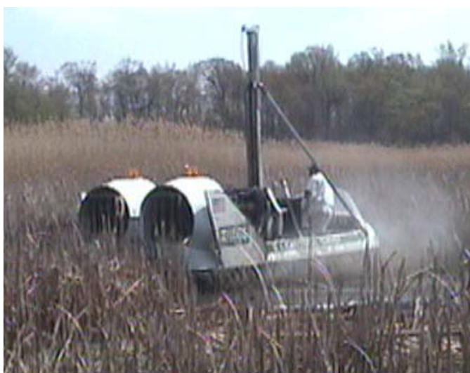
Figure 4.9. Vibracore systems used at the West Branch Canal Creek wetland site at Aberdeen Proving Ground, Maryland. A. portable hydraulic unit with vibration only. B. portable hydraulic unit with vibration and hammer action. C. Hoverprobe with attached hydraulic vibracore unit with vibration only.
