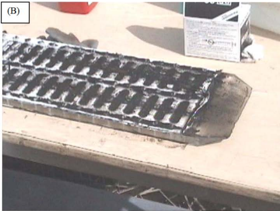
Figure 3.5. Photographs showing (a) removal of a peeper from the wetland sediment and (b) close-up view of peeper prior to sampling.
