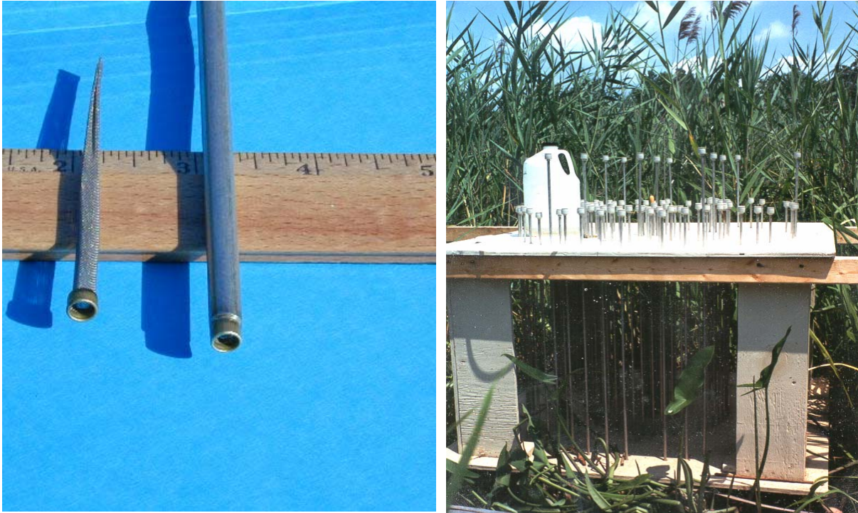
Figure 4.21. Photographs of (a) tubing and screen components of tubing sampler and (b) tubing sampler array at wetland field site. This extensive tubing sampler array was used for a detailed ground-water tracer study.
