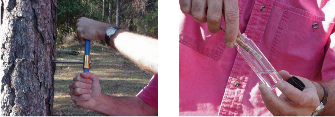
Figure 4.11. Illustration of tree core sampling procedure for analysis of chlorinated volatile organic compounds: (a) tree coring using standard forestry coring device, and (b) addition of core to vial containing methanol for extraction.
