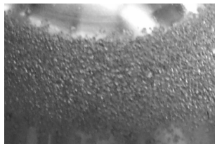
Figure 7. Type 304 stainless steel electrode following 250,000 shots with original oil flow configuration. Width of the arc band ~ 1.7 cm.
