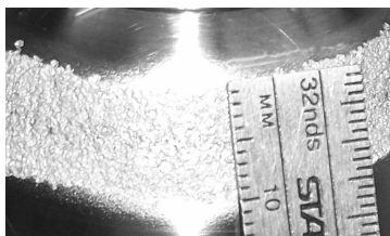
Figure 9. Second type 304 stainless steel electrode after 150,000 shots with enhanced oil flow configuration. Width of the arc band ~ 1.0 cm
