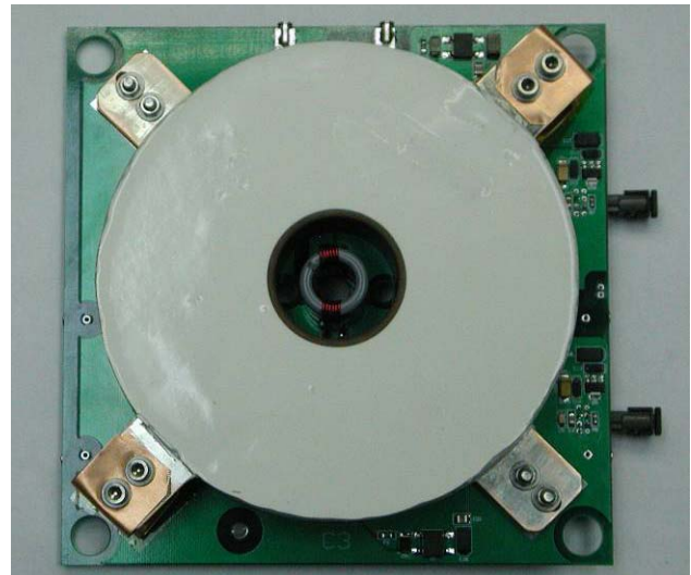
Figure 3. Back view of a single modulator board showing the stage capacitor and utility power system.
