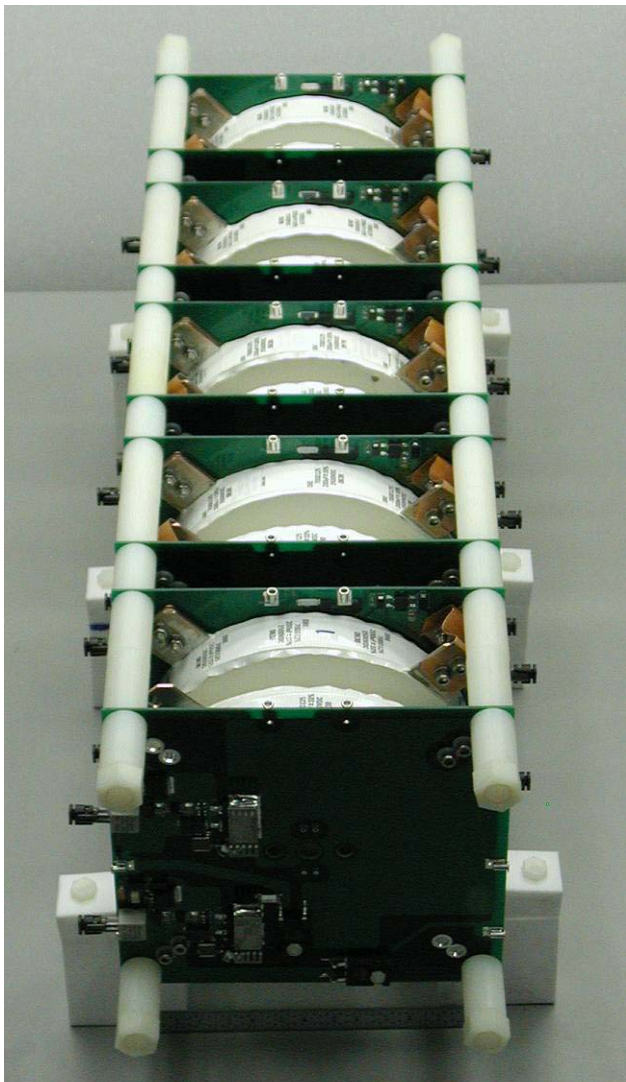
Figure 4. The scaled prototype modulator is a stack of 10 solid-state modulator stages each laid out on their own circuit board. the modulator operates at 1300V per stage for a pulsed output voltage of 13 kV.
