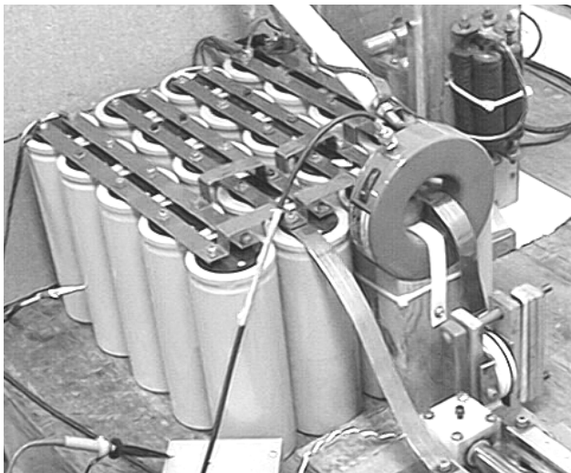
Figure 3. The PFN and thyristor used to power the HCEL.
