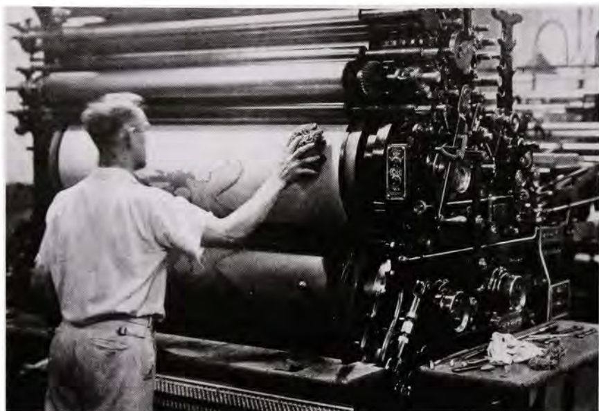
76. U.S. Lake Survey pressman Erich Rhode cleaning the 38 × 52 inch Potter offset press, Federal Building, Detroit, 1937. Courtesy, U.S. Lake Survey Installation Historical Files, National Ocean Survey.
