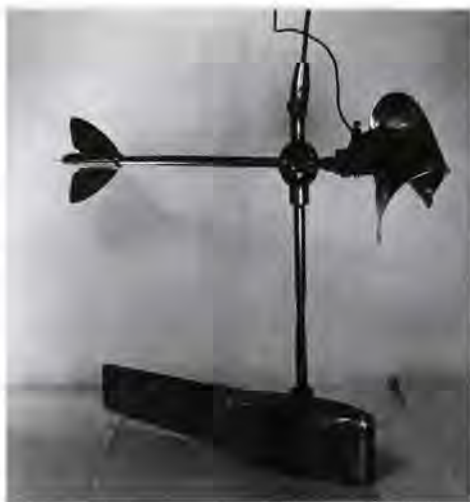
38. U.S. Lake Survey current meter used for measuring river discharge flow. Courtesy of the Detroit District, Corps of Engineers.
