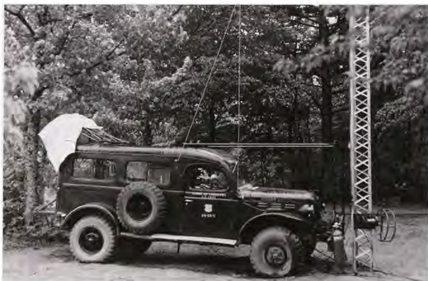
53. U.S. Lake Survey field party truck housing SHORAN instruments with telescoping tower, northern Michigan near Lake Superior, 1958. Courtesy, U.S. Lake Survey Installation Historical Files, National Ocean Survey.
