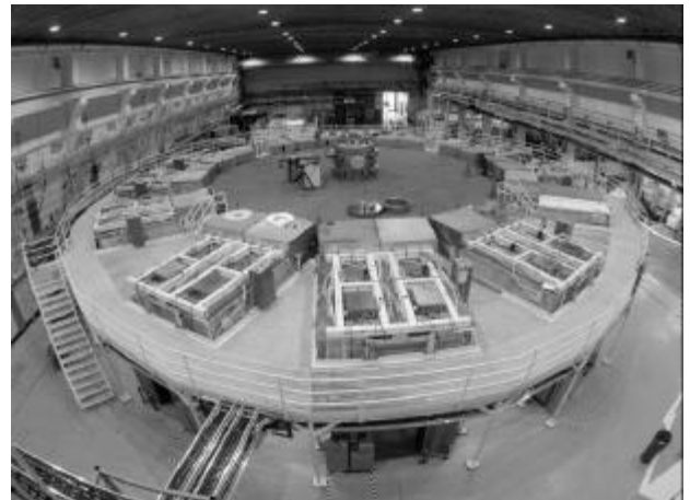
Figure 1. The Atlas generator consists of twelve capacitor bank tanks surrounding a central target chamber.
