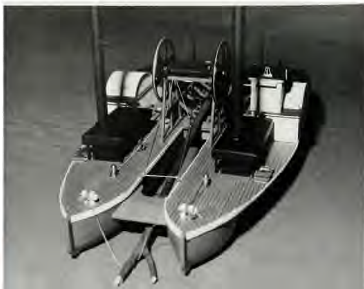
ILLUSTRATION 22. This model of Shreve's snag boat, the Archimedes clearly illustrates the design of Shreve snag boats. Shreve used the Archimedes in clearing both the Red River and the Arkansas River during the 1830s.
