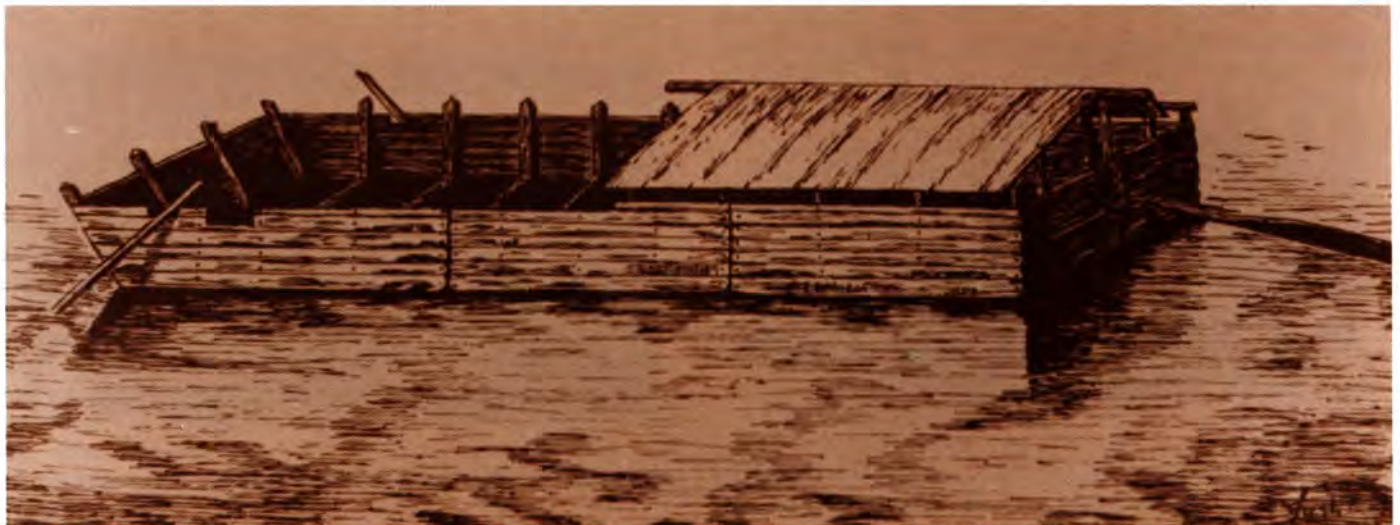
ILLUSTRATION 16. A sketch of the type of flatboat used on the rivers of the Arkansas, White and Red River Basins
