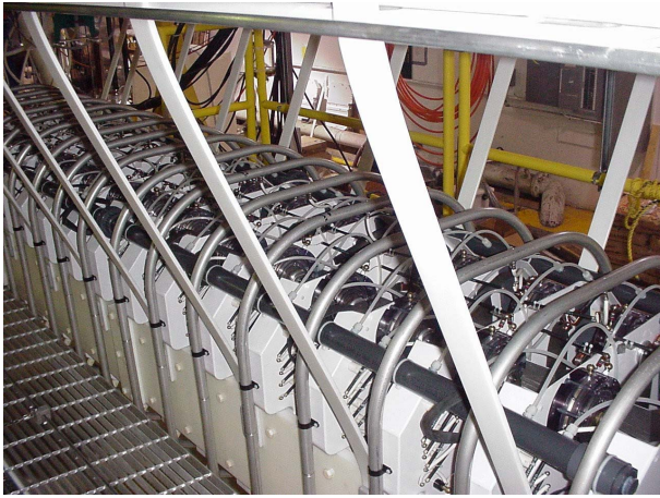
Figure 2. Cygnus Marx Generator on nylon straps.
