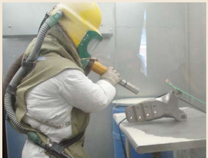
Based on participants' comments and results from the NDCEE demonstration, RDECOM's Aviation Engineering Directorate released an MEO on July 24, 2008, that allows CCAD to use CHP on aviation airframes. Photo shows a CCAD blaster using the CHP technology on a UH-60 Blackhawk rotor blade cuff.
