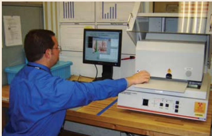
XRF technology, transitioned to Tobyhanna Army Depot after a successful NDCEE demonstration, helps the DoD manage lead-free components and materials in its supply chain.
