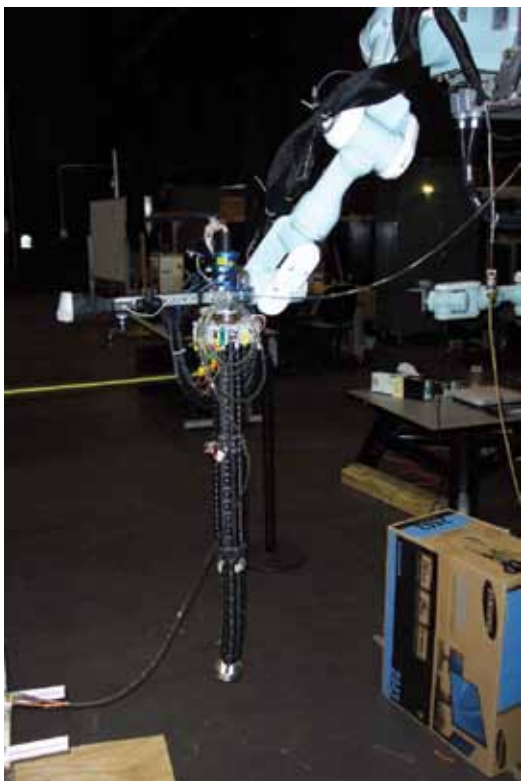
FIGURE 9 The combined robotic refueling system, including the PA10 and Octarm.
