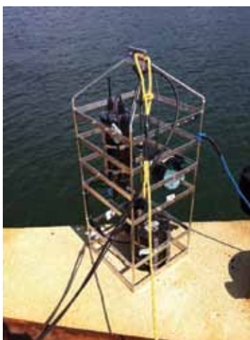
Moored and autonomous underwater vehicle (AUV) deployment of immunosensor systems.
