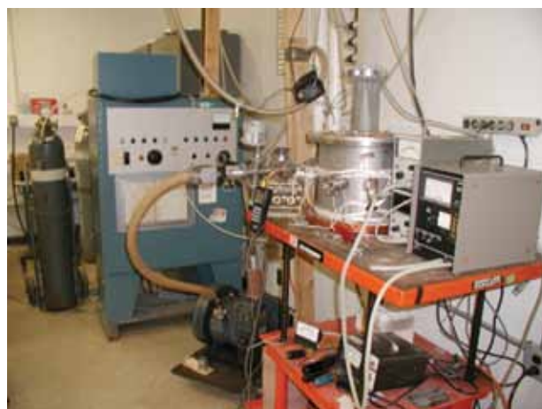
(b) FIGURE 10 (a) Schematic and (b) photograph of the NRL 6 kW, 2.45 GHz microwave system for titanium sintering experiments.
