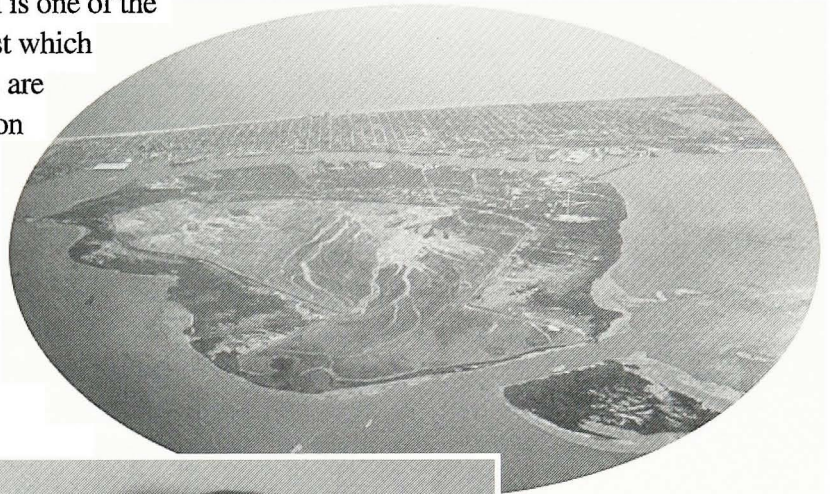
Pelican Island, shown in the above photo, was largely built from material dredged from the ship channel.
