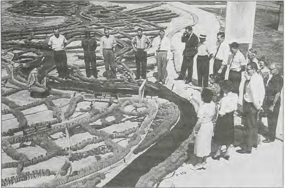
A guide at the Waterways Experiment Station explains the model of the Old River area and the plans to prevent the Atchafalaya from capturing the Mississippi. The model was built in 1936 with a vertical scale of 1:100 and a horizontal scale of 1:2,000. Photograph c. 1960.
