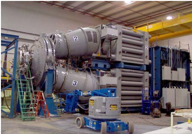
Figure 1. Decade Quad machine presently on the floor at the DRTF. A second "quad" will be added before 2007.
