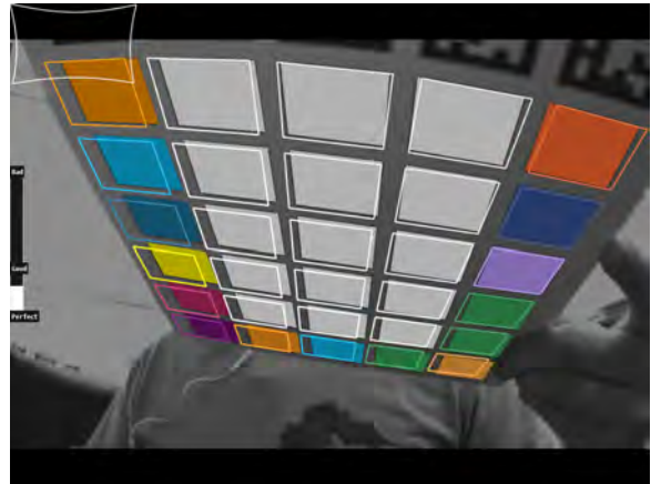
Fig. 1: The AprilCal GUI. Our system combines the ability to reason about unseen targets and a novel quality metric to make suggestions to the user about where to place the target. The user is notified that calibration is complete once the desired accuracy has been reached, typically achieving < 1 pixel of error after 6-8 images.
