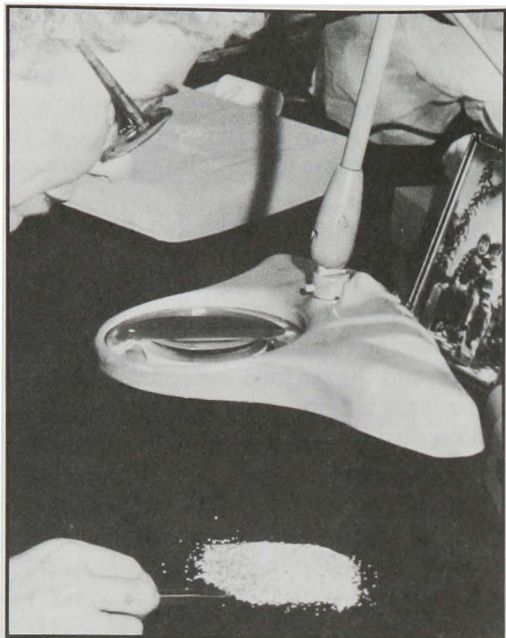
Specialists at the Southwestern Division Laboratory sort and grade industrial diamonds for use in drill bits.
