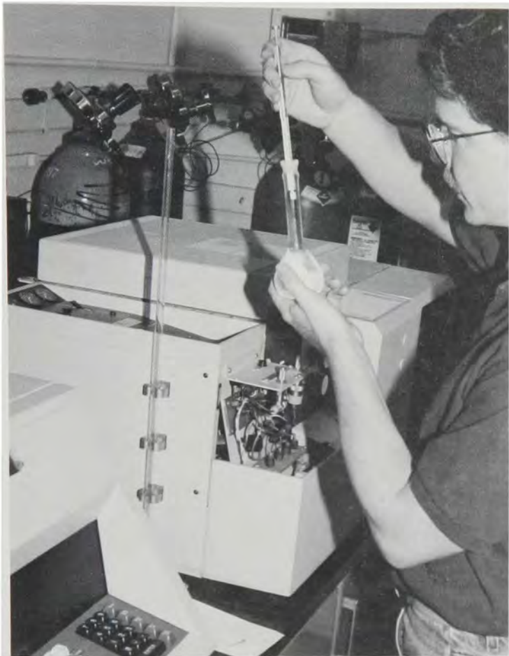
A technician at the Southwestern Division Laboratory prepares a sample to be analyzed in the gas chromatograph for organic substances such as pesticides.
