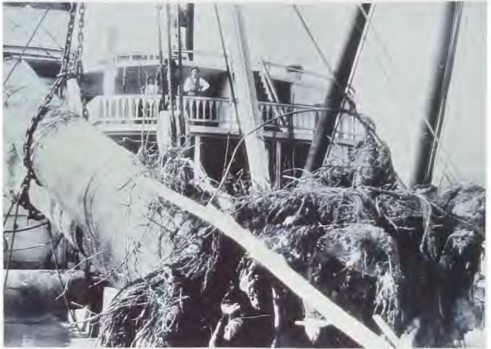
Logjams on the Trinity River in Texas prevented navigation in spite of constant work by snag boats like this one.
