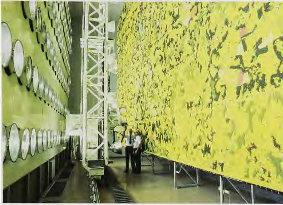
Floodlights (left) illuminate terrain (right) in this helicopter flight simulator at Fort Hood.
