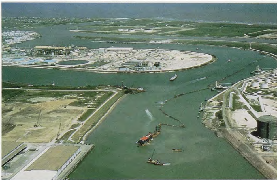
This broad basin in Freeport Harbor, Texas, lets large ships turn around.
