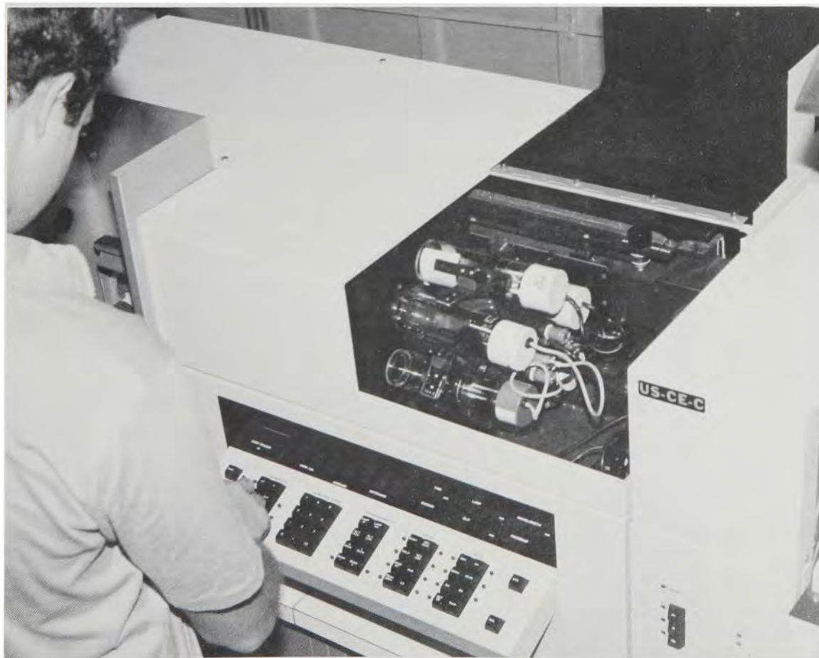
The atomic spectrophotometer at the Southwestern Division Laboratory can determine the amount and type of heavy metals in a prepared sample.
