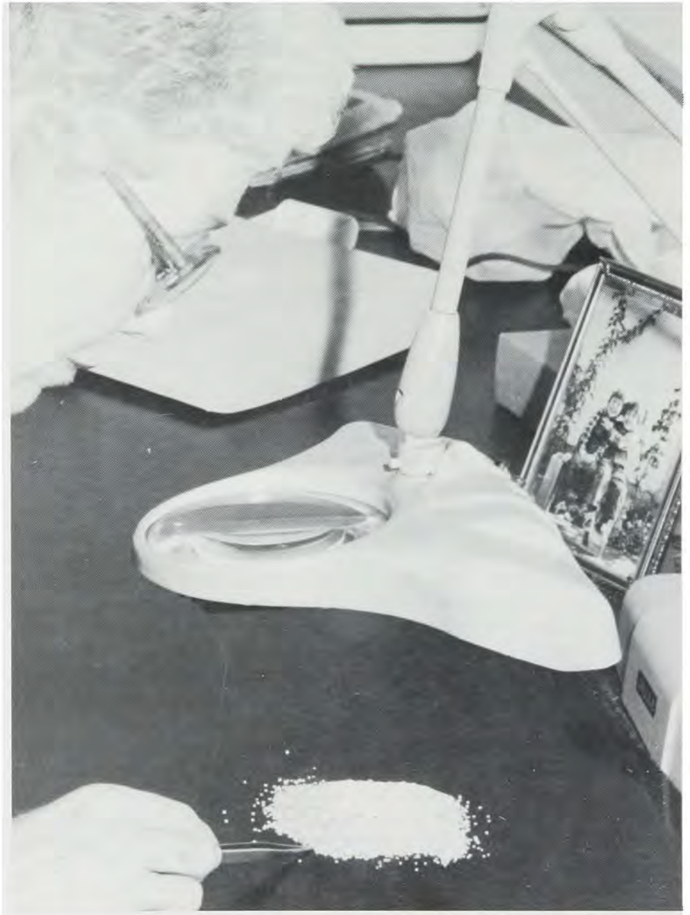
Specialists at the Southwestern Division Laboratory sort and grade industrial diamonds for use in drill bits.
