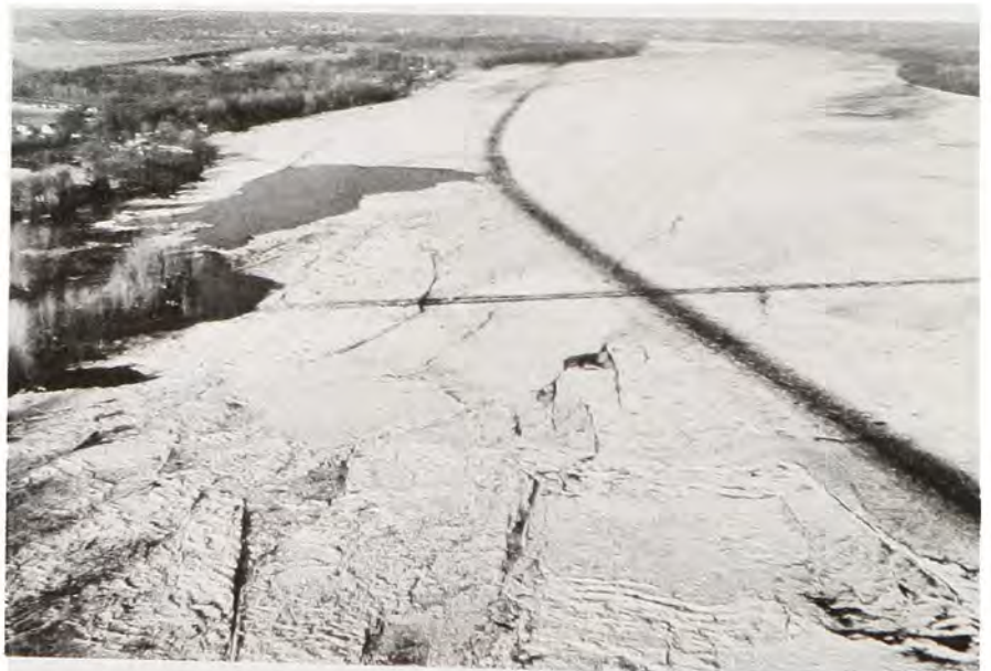
One of the worst ice jams on the Mississippi occurred in February 1966. The dark strips on the ice are coal dust, dropped from a plane by the Corps of Engineers in an experiment to hasten melting.
