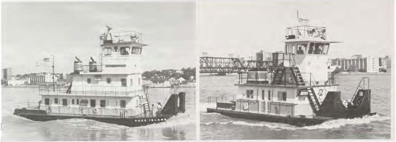
The diesel towboat Rock Island , 64 feet long with 850 horsepower.
