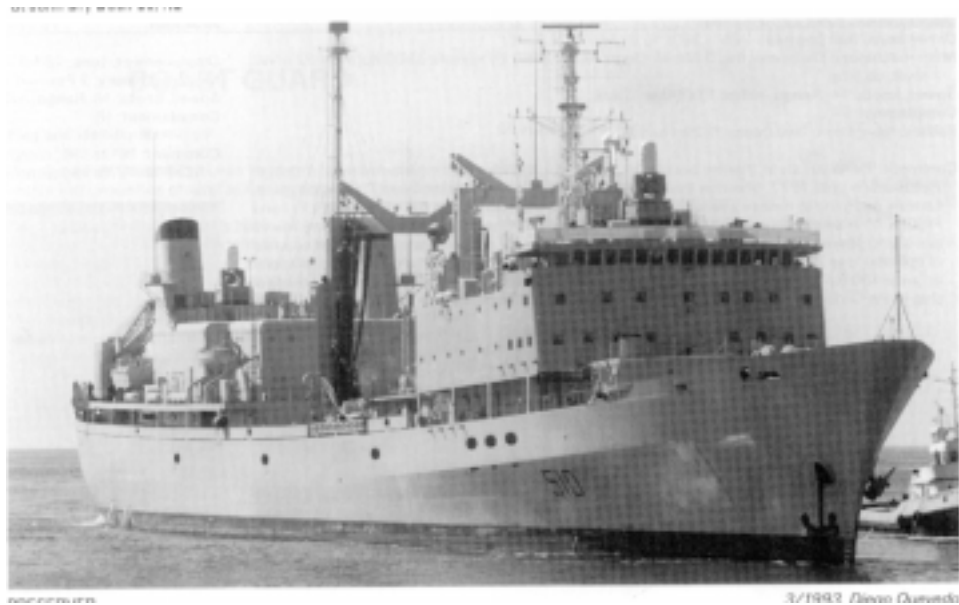
Figure 3.5: Application of a Stayed Polemast Structure
