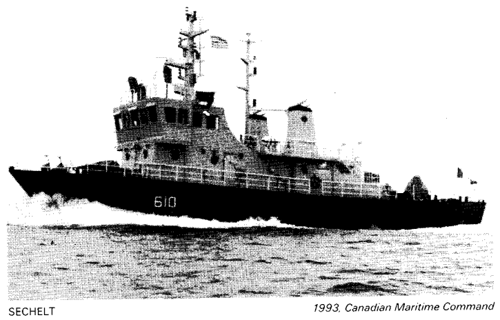
Figure 3.3: Application of Unstayed Polemast Structures on Canadian Ships (a) Pierre Radisson, (b) Sechelt
