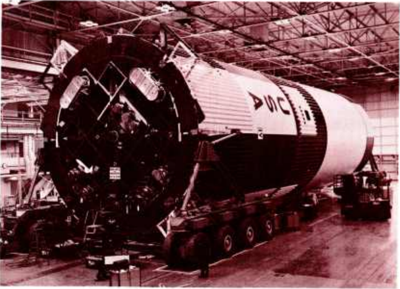
FIGURE 115 First stage, Saturn V, showing thrust structure
