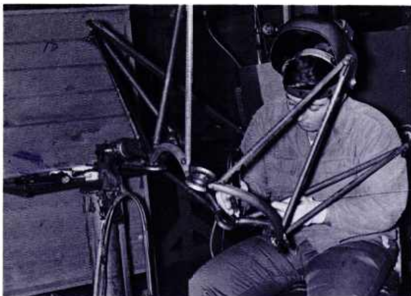
FIGURE 99 Welder completing engine mount
