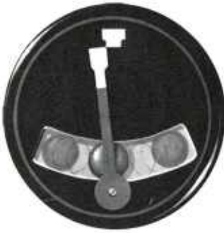
FIGURE 133 THE TURN-AND-BANK INDICATOR, FORMERLY REFERRED TO AS "NEEDLE & BALL"; OPERATES LIKE A CARPENTER'S LEVEL: WHEN BALL IS IN THE CENTER, PILOT IS EITHER FLYING STRAIGHT AND LEVEL OR MAKING A WELL CO-ORDINATED TURN: NEEDLE TELLS HIM WHICH: IF AIRCRAFT IS TURNING TO RIGHT OR LEFT, NEEDLE MOVES TO THE RIGHT OR LEFT.
