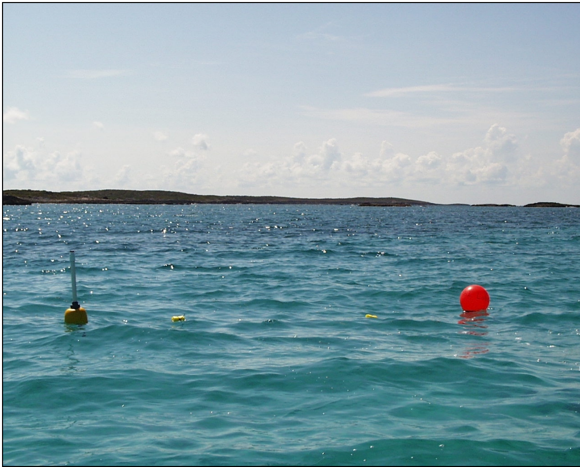
Figure 2. Photograph of the fiber-optically tethered surface buoy which measures remote-sensing reflectance. The HydroRad to which this buoy is tethered is mounted on the bottom (see Figure 1), where it also measures bottom irradiance reflectance simultaneously with the remote-sensing reflectance measurement.
