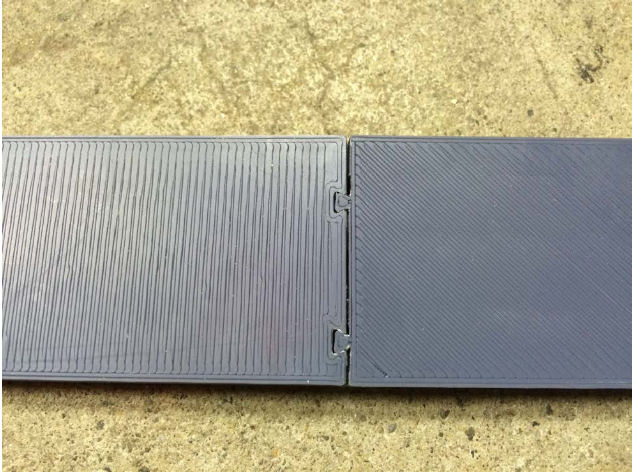
Figure 25: Finishing and deburring of the interlocking features was required to facilitate model connection.
