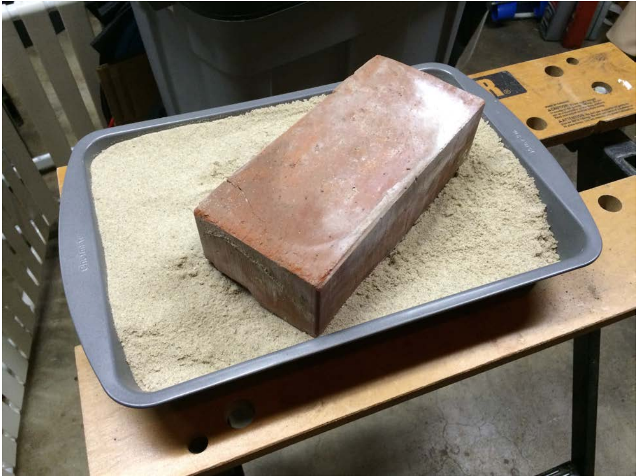
Figure 22: Warped parts were annealed under a weight in a bed of sand to control heat transfer rate and ensure uniform cooling.
