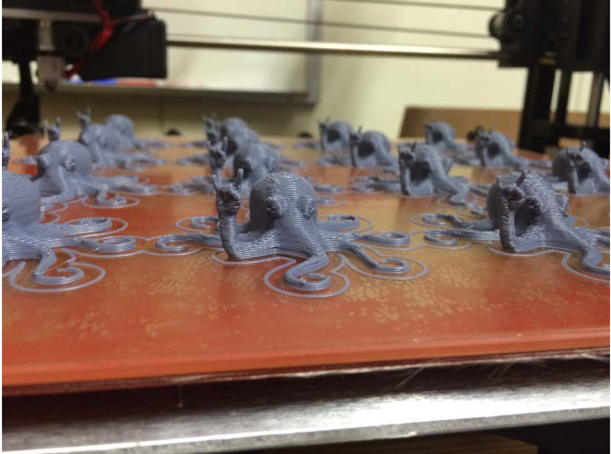
Figure 51: The batch print operation of the "Rocktopus" model revealed that each instance showed minor variation based on extrusion start/stop points.
