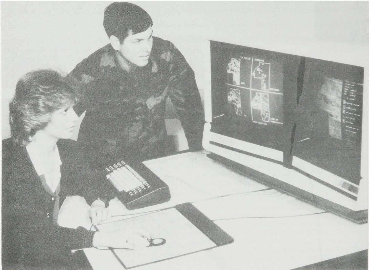
A USAETL scientist demonstrates a Digital Topographic Support System (DTSS) interactive work station, used to develop and evaluate automated terrain analysis software.
