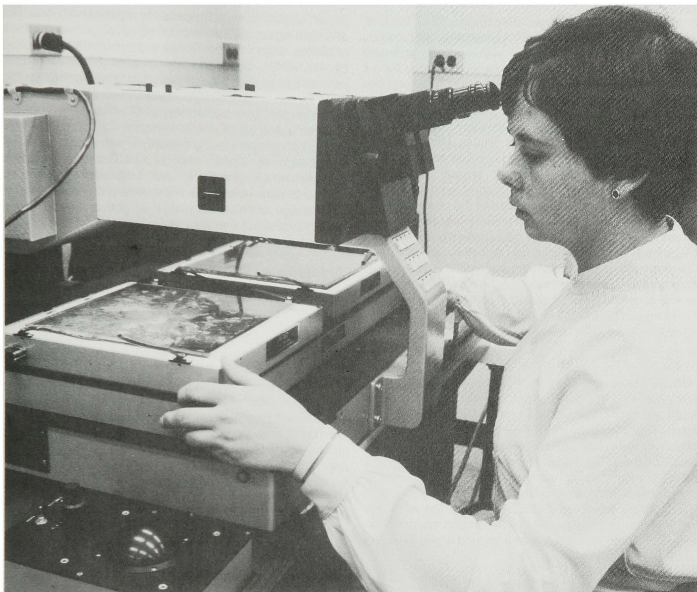
A scientist prepares to view stereopairs on the Computer-Assisted Photo Interpretation Research (CAPIR) system.
