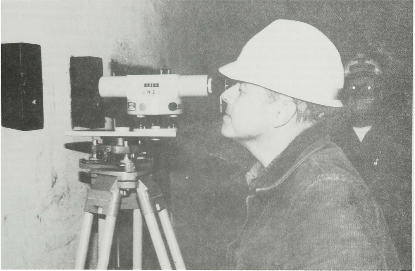
Using mirrors, a USAETL scientist measures the degree of tilt of a dam wall.
