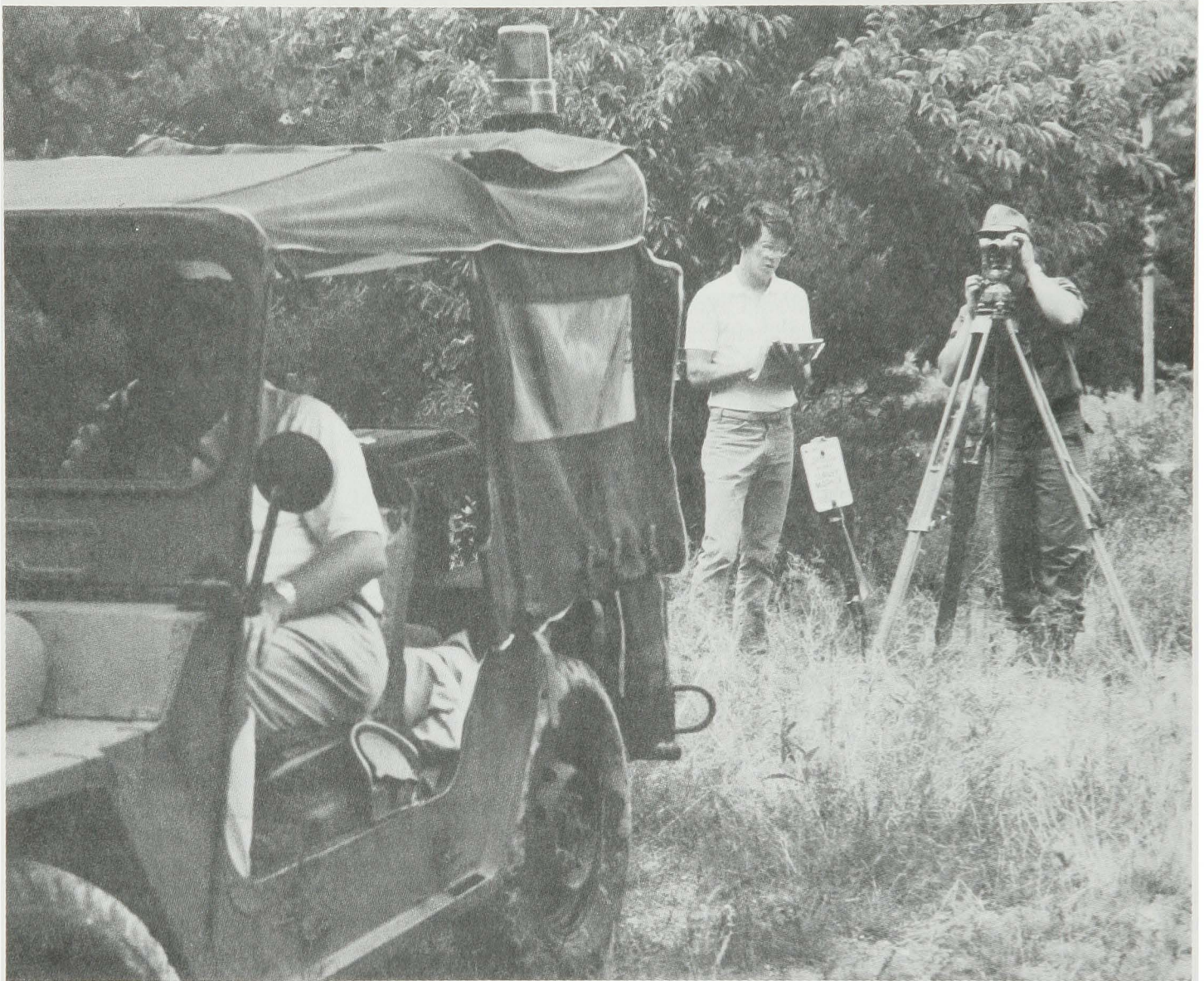
Scientists record a survey position to give the Position and Azimuth Determining System a point of reference.
