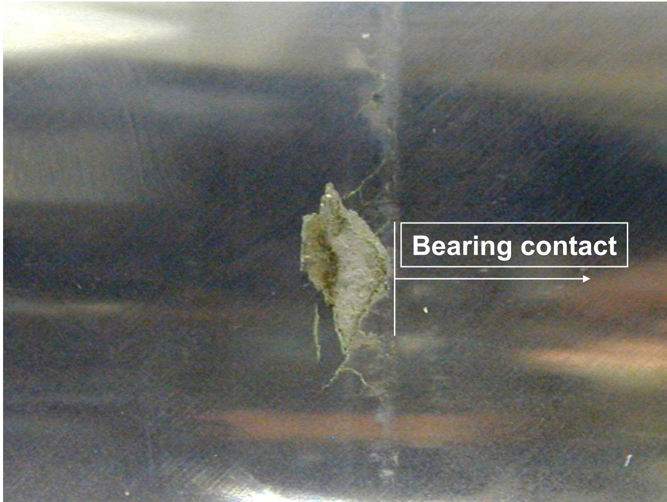
HVOF COATING AFTER 570,00 CYCLES
