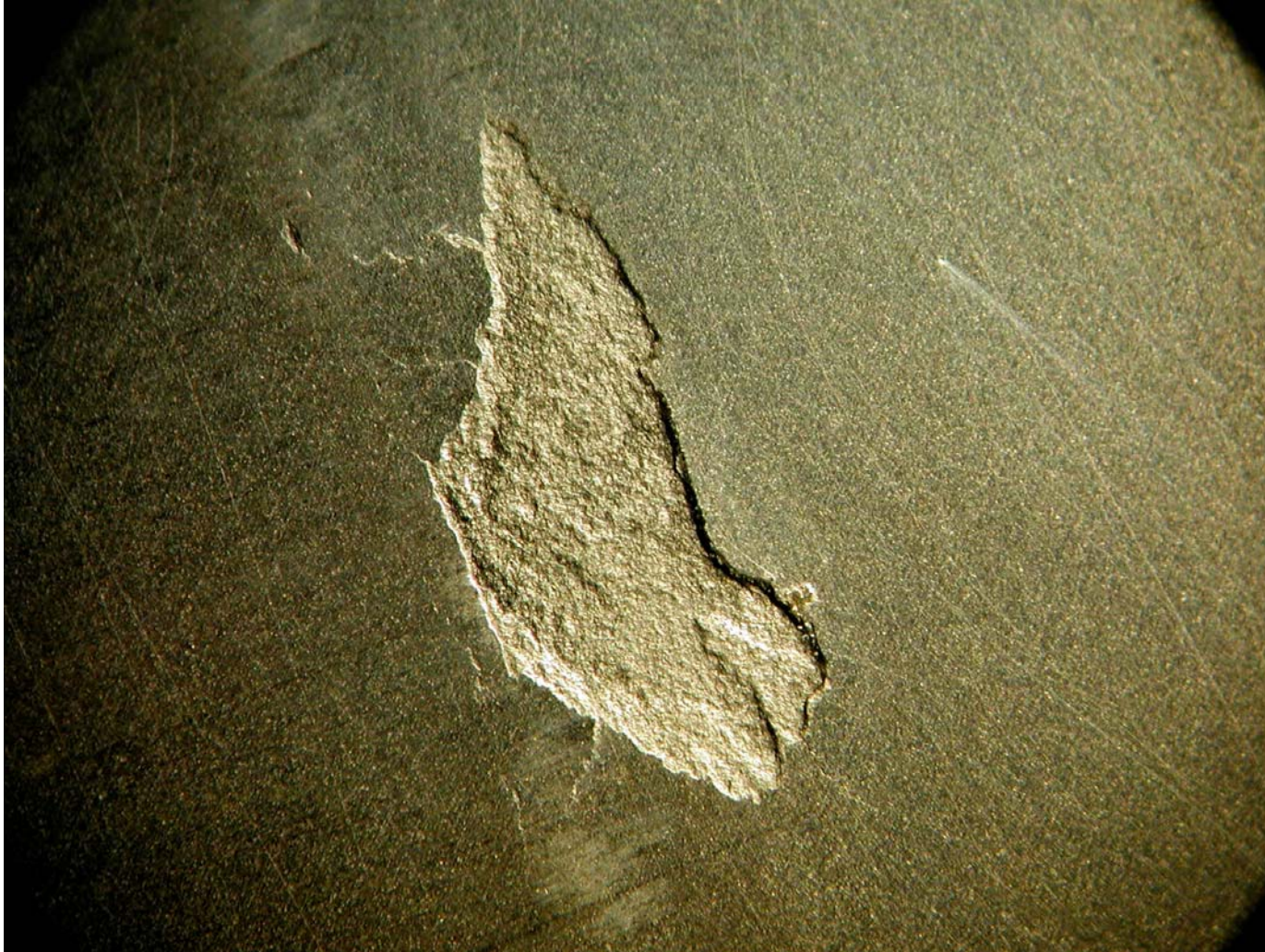
HVOF COATING AFTER 285,000 CYCLES
