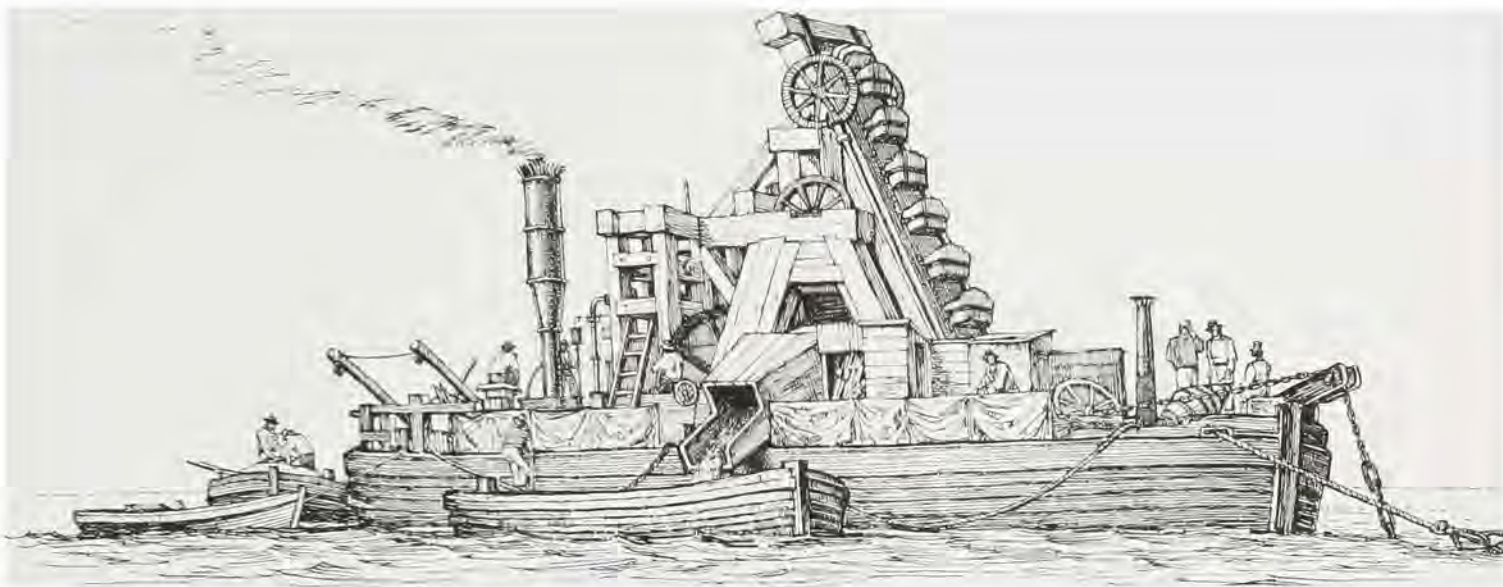
The mud dredger of the 1830's was best exemplified by the steam-driven endless chain bucket or ladder dredge. This type retained the favor of the Europeans, but was replaced in American waters by grapple and dipper dredges.
