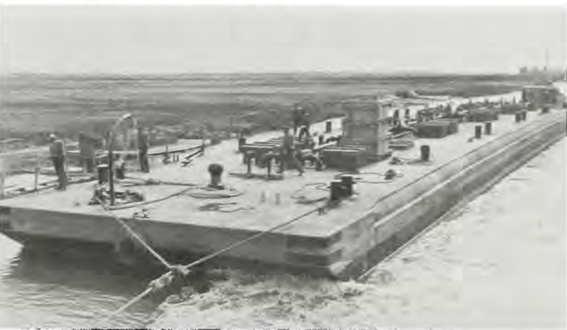
The concrete barge, being towed through the Lewes Canal. The barge measured 195 feet in length by 35 feet in breadth, drew 11 feet of water and displaced 850 DWT. Built in sections which were later joined together, the weight of the reinforcing steel proved so great that the vessel bowed amidships from the strain.
