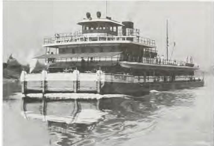
Steel Hull 2000 H.P. Twin Screw Towboat, Midway Islands. Measured 180 feet in length by 52 feet in breadth, with a draft of 11 feet. Shown in bow view immediately after a complete 180 degree turn at 185 RPM.
