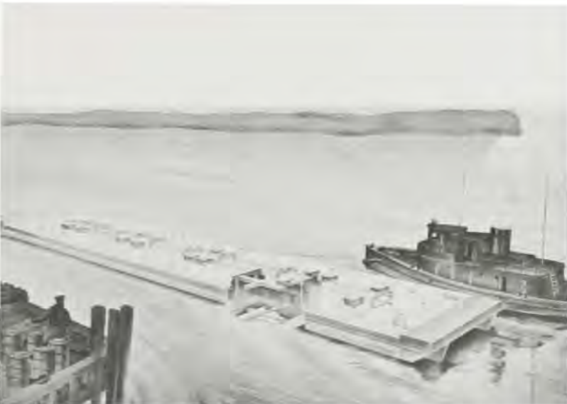
Artist's conception of an experimental concrete oil barge, with cutaway depicting steam piping required to heat the viscous crude oil.
