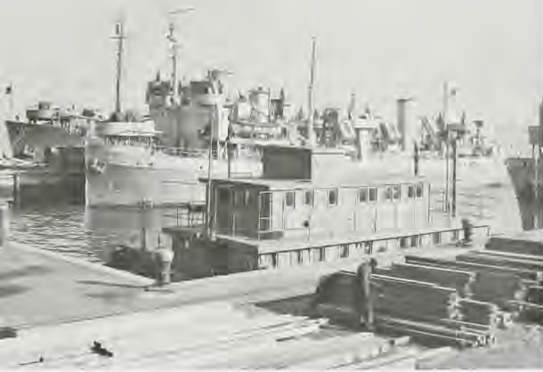
The dredges Chester Harding and William T. Rossell at Fort Mifflin. December 1943. Among the dredges militarized by the Philadelphia Engineer District, these vessels were provided with 3-inch deck guns, as well as 20 mm anti-aircraft guns.
