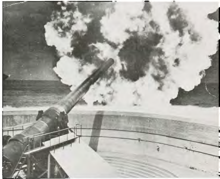
The Model 1895 12-inch rifle was 37 feet long, and could fire a 900 pound steel shell approximately 29,000 yards.
