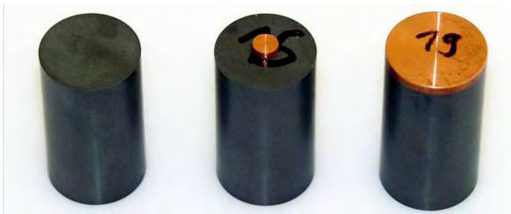
Figure 4. Three different target configurations: bare, small Cu buffer, and Cu cover plate.
