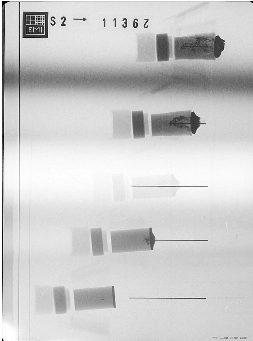
Figure A-23. X-ray picture for Exp. 11362: cover-plate SiC, v_p = 1612 m/s.
