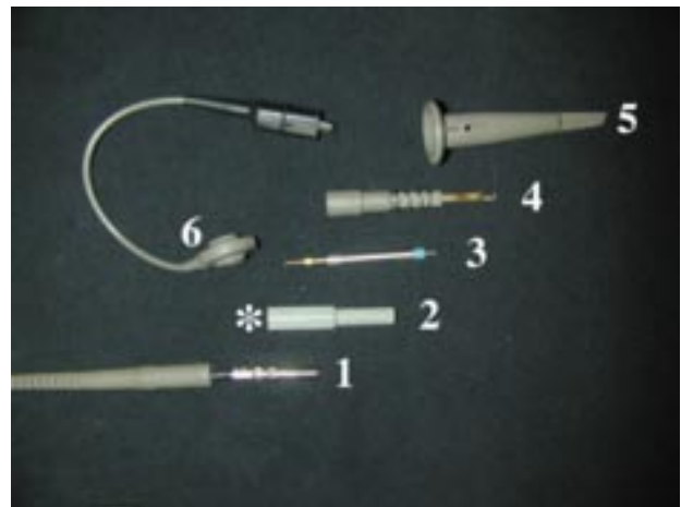
Figure 2. Parts from a Tek. P6139A probe. Refer to numbered parts for assembly procedure.
