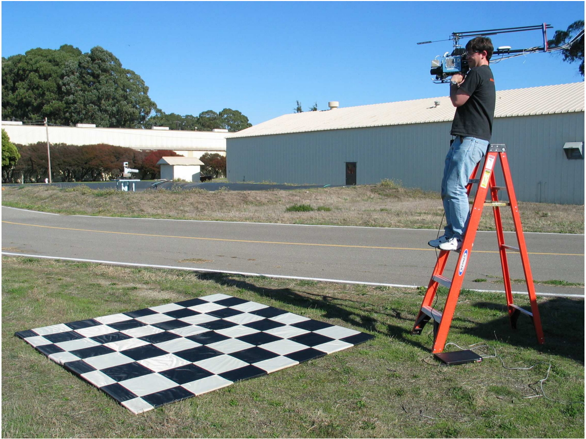
Figure 6.5: Camera to GPS/INS calibration. Courtesy of David Shim.
