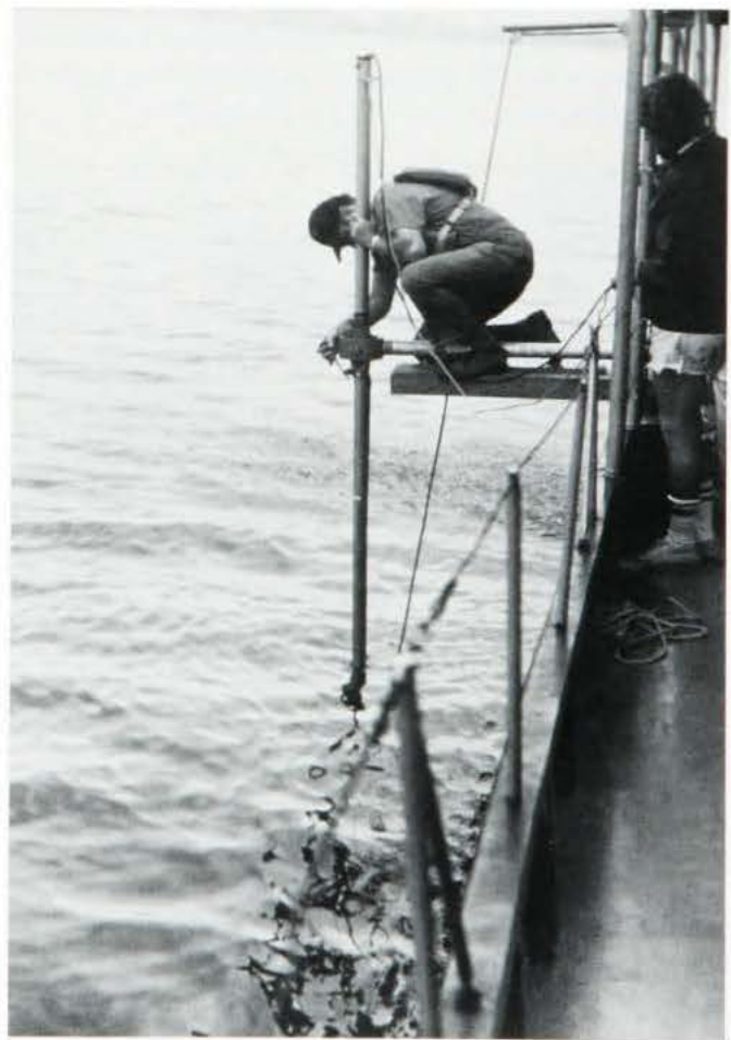
CERC Employee Setting a Wave Gage
