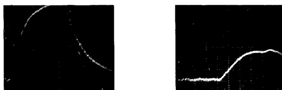
A. Voltage Measurement Across a 6 \Omega load, 3340 V/div; 50 ns/div. B. Current through a 6 \Omega load, 1000 A/Div; 50 ns/div.
