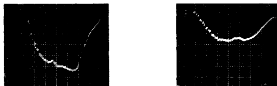
A. Voltage Measurement Across a 6 \Omega load, 3340 V/div; 50 ns/div. B. Current through a 6 \Omega load, 3340 V/Div; 50 ns/div.
