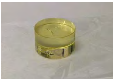
Fig. 3. Billets of GPGN glass
